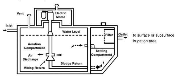
Figure 2: Diagram of typical aerobic treatment unit (without effluent disinfection)
