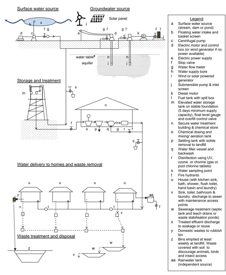
Figure 1 - Typical water supply and waste management system for small communities
