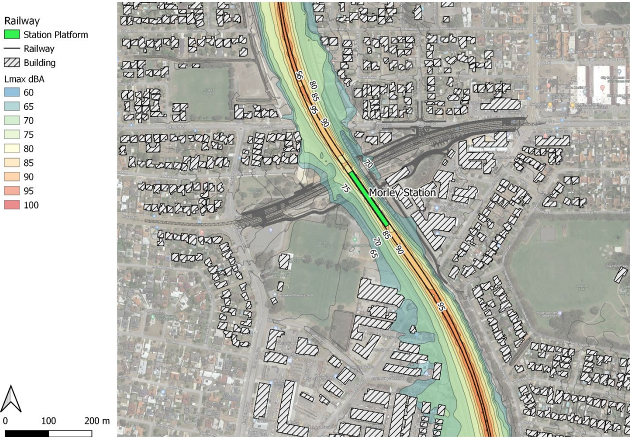
Figure 9: Forecast distribution in airborne noise from rail operations for comparison with L_{Amax} criteria
