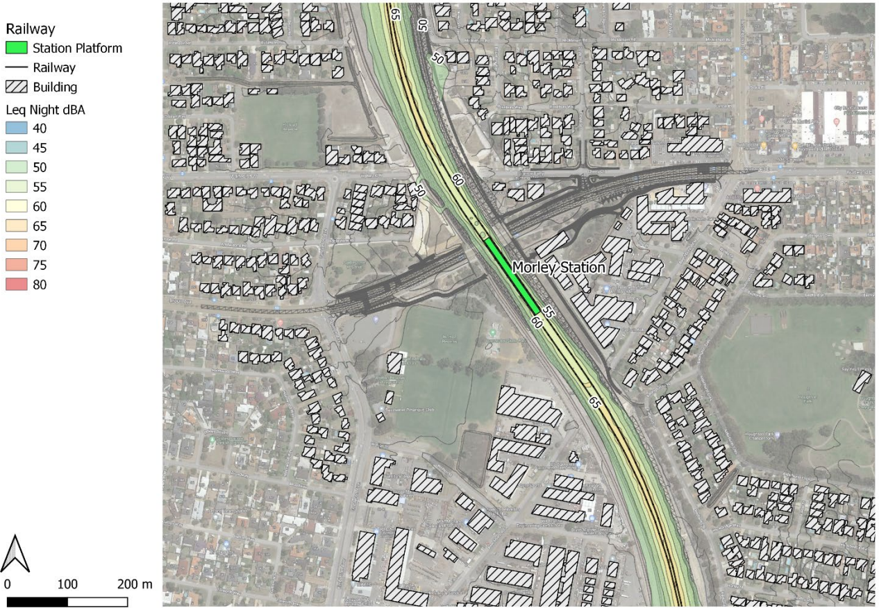
Figure 8: Forecast distribution in airborne noise from rail operations for comparison with L_{Aeq} night criteria
