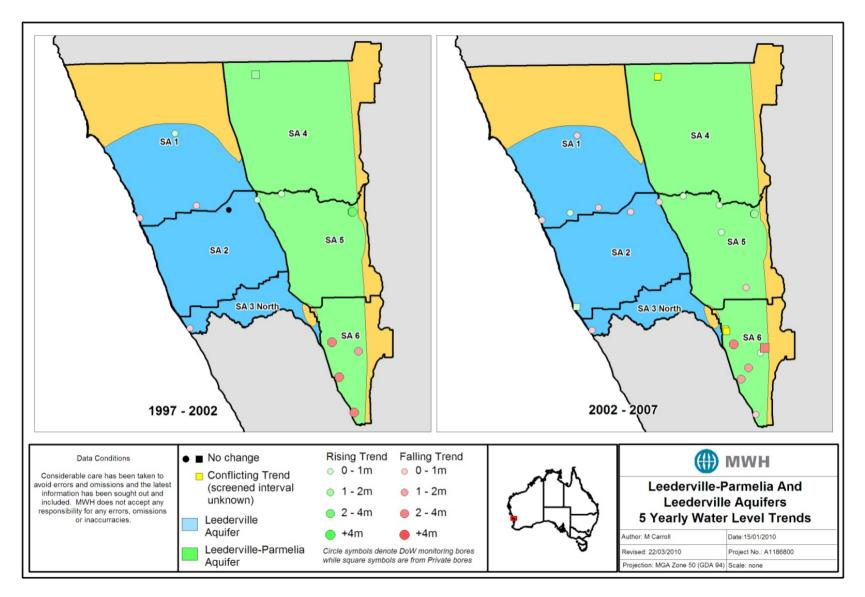
Figure 15 Groundwater trends within the Leederville and Leederville-Parmelia aquifers (MWH 2010)
