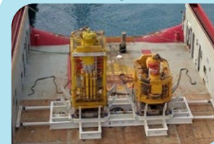
MISSION DECK™ No weld sea fastening system for rapid logistics on vessels of opportunity in "one tide".
