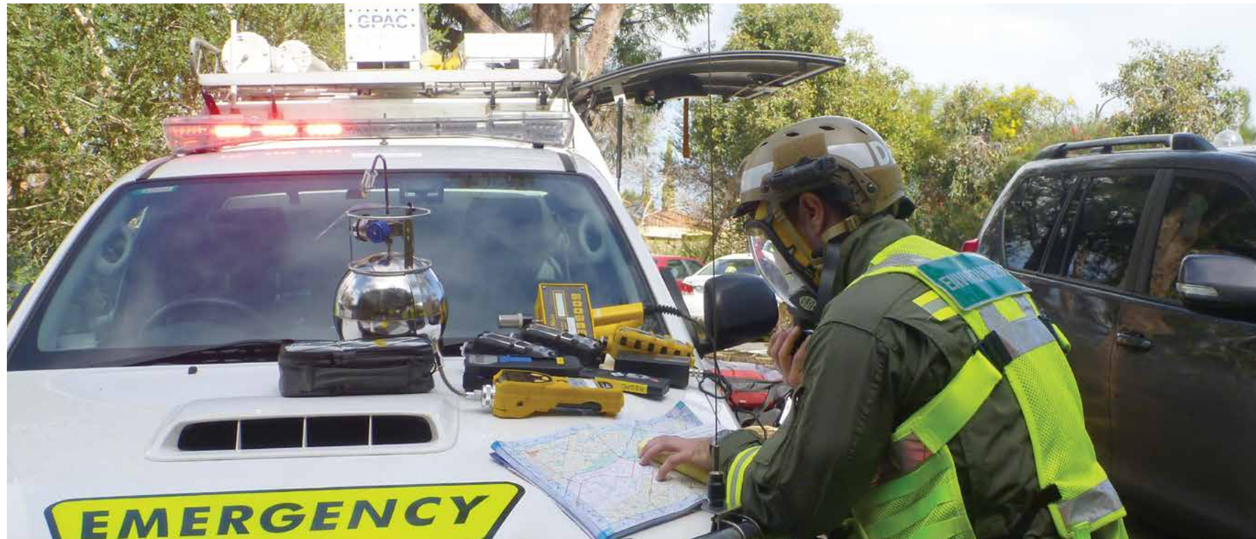
Figure 5.9 – Pollution Response Vehicle showing its GPAC video and chemical real time data system and chemical detecting
