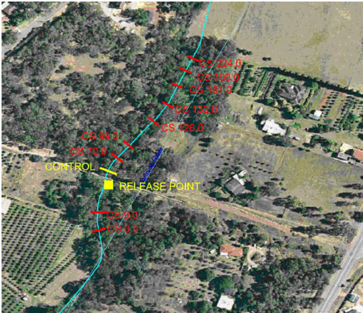
Figure 13 Aerial view of Bernard Street management reach showing the cross-sections, control point and release point
