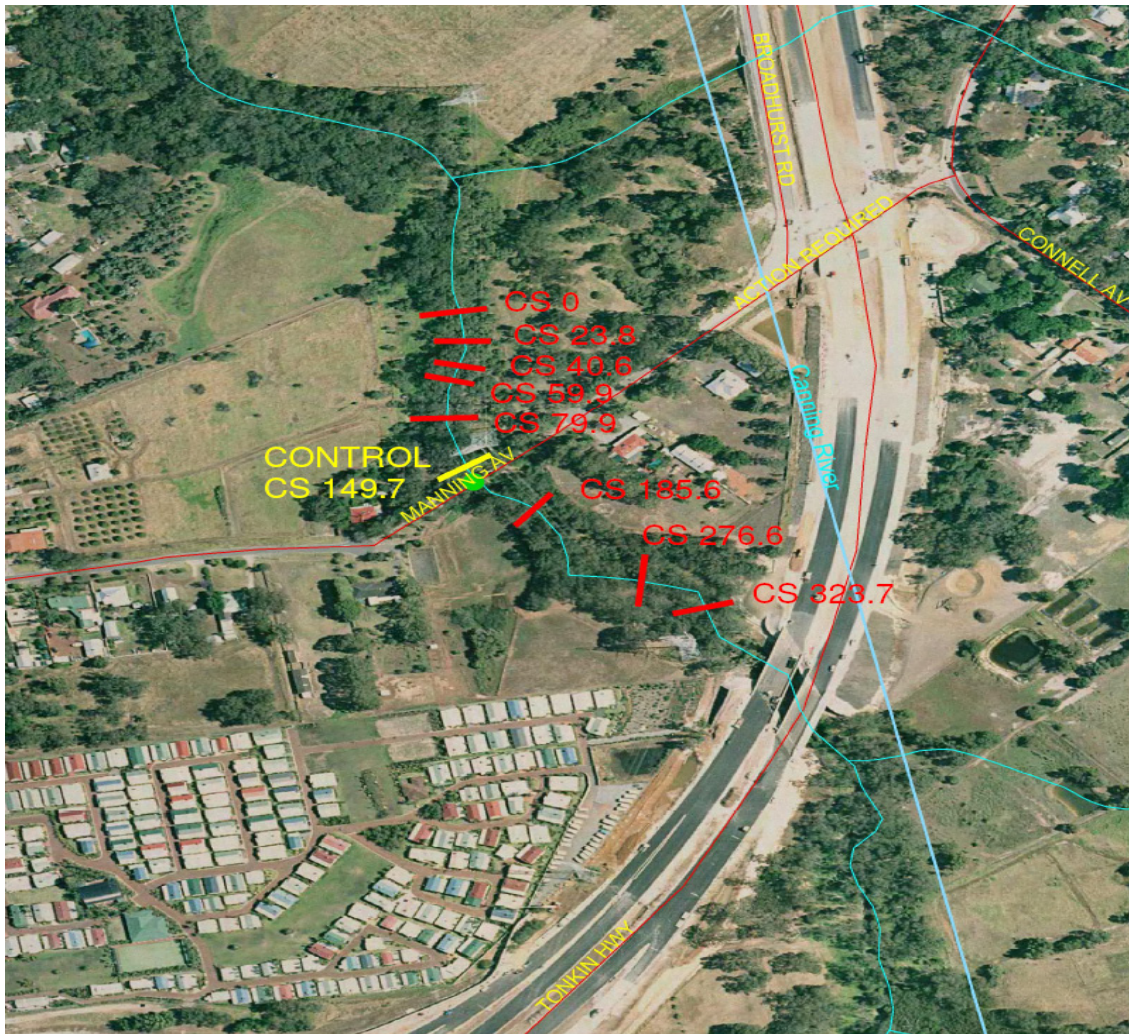
Figure 19 Aerial view of Manning Avenue management reach showing the cross-sections, control point and release point
