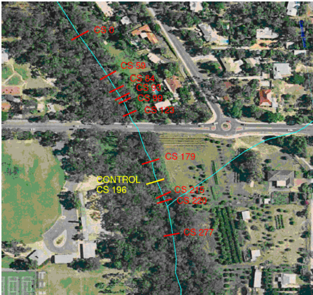
Figure 16 Aerial view of Orlando Street management reach showing the cross-sections, control point and release point
