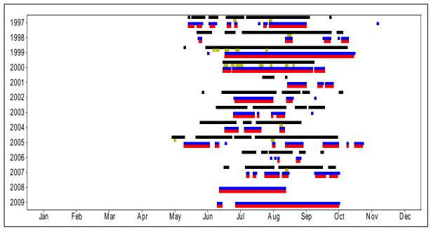
Legend – modelled EF regime (red bars), 'undammed flow' (black bars), 'catchment flow' (yellow bars), 'current flow' (blue bars)
