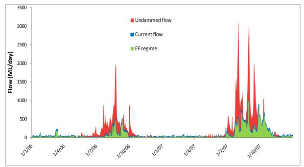
Figure 20 Daily flow in 2006 and 2007 for 'undammed', 'current' and 'EF' regime showing the difference between the flow regimes.
