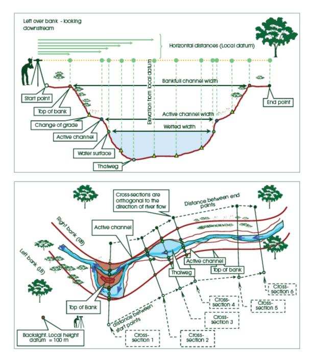
Figure 8 Schematic diagram of a river reach. The upper diagram shows the point data surveyed as part of a cross-section. The lower diagram shows the longitudinal layout of cross-sections along a river reach.
