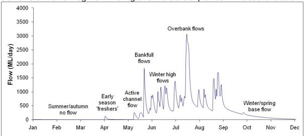
Figure 6 Representative hydrograph of a typical South West stream with different flow components labelled
