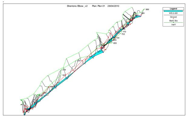
Figure 9 Structure of the HEC-RAS hydraulic model for the representative study reach (Shentons Elbow reach) in the lower Collie River. The blue trace shows the water level at the time of the channel surveys.
