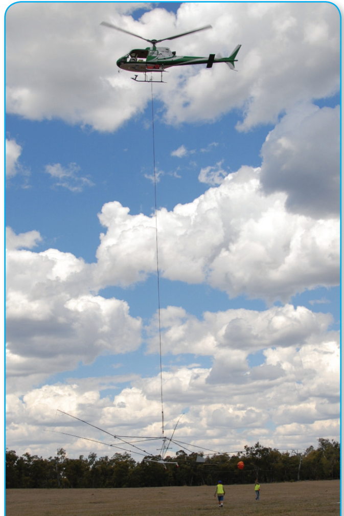
Helicopter lifting off at a test site near Chittering with towed device designed for electromagnetic surveying. (Photo courtesy of GPX Surveys)
