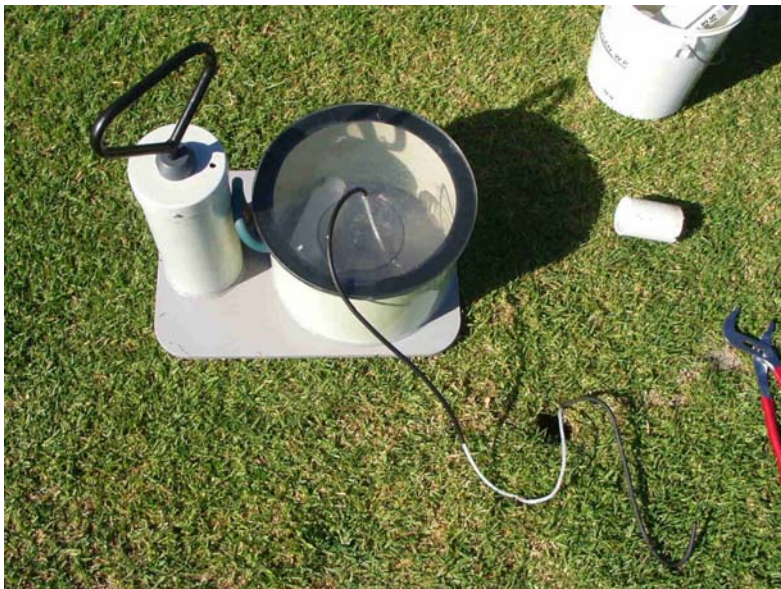
Figure 3. Field sampling apparatus (suction pump) used to sample buried lysimeters with sampling and breather tube emerging from the established turf.
