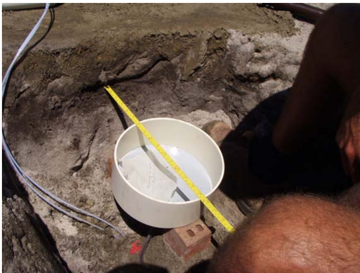
Figure 1. Soil leachate lysimeter being installed and levelled.
