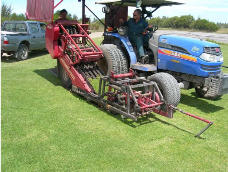
Figure 9. Harvesting of the turf using a tractor-mounted harvester.
