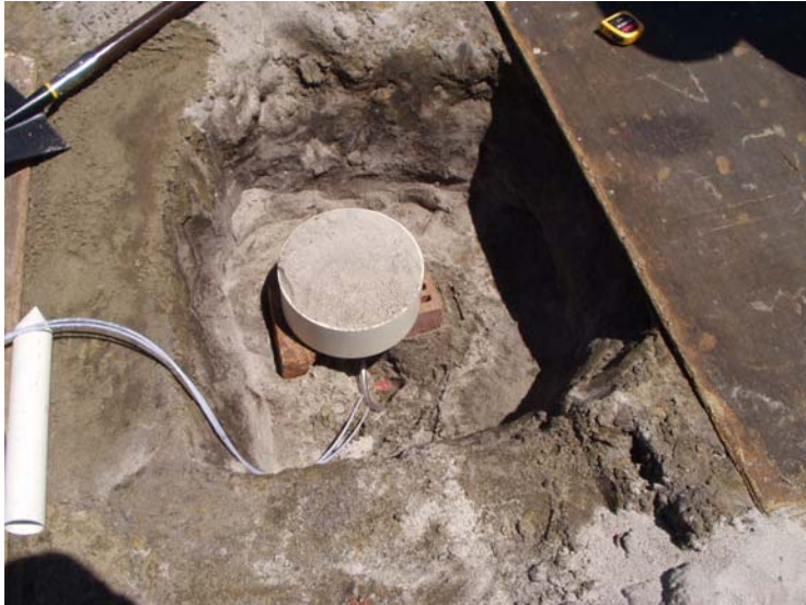
Figure 2. Lysimeter being installed and packed with local sandy soil.
