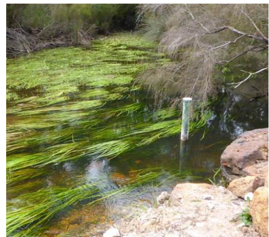
Manjimup Brook outlet temporary gauging station - 100mm PVC slotted housing with pressure probe (for water level) recording instrument
