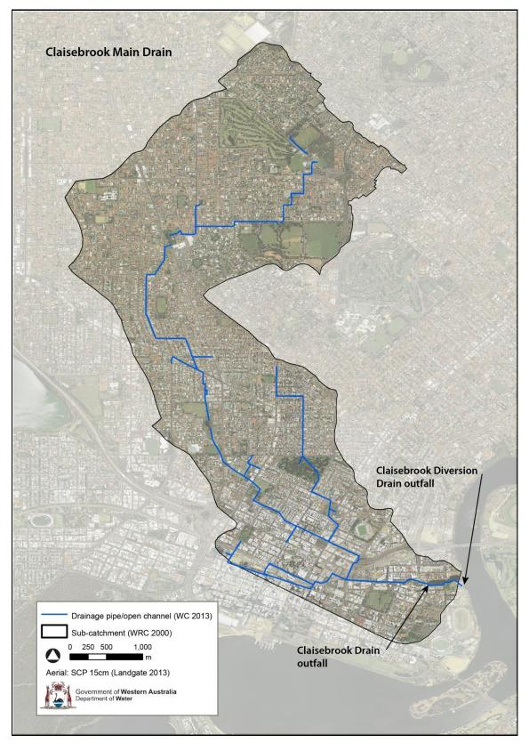
Figure 24 Drainage map of the Claisebrook Catchment.
