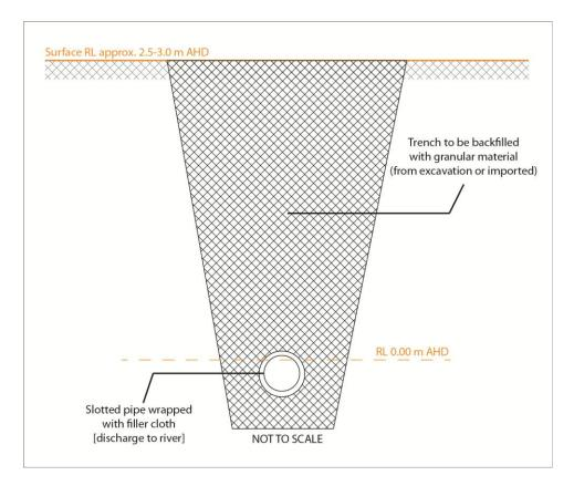
Figure 21 Groundwater interception drain (GID) in cross-section; RL: relative level; AHD: Australian Height Datum (modified from Tingay and Associates 1994b).
