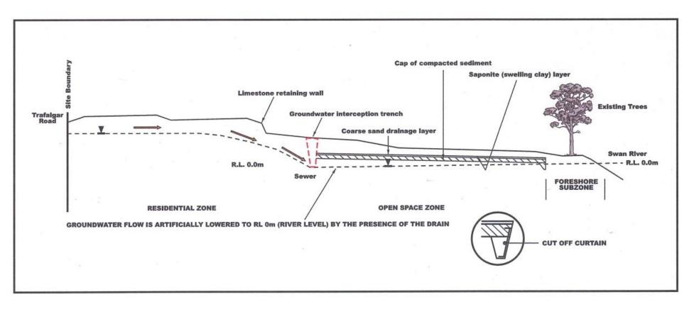
Figure 23 Schematic representation of function of containment area showing cut-off curtain, groundwater interception drain and capping layer (source: ENV 2011a).
