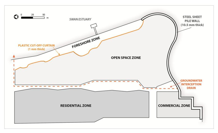
Figure 20 The containment Cell. Comprising plastic cut-off curtain, steel cut-off wall and groundwater interception drain (modified from ENV 2009).
