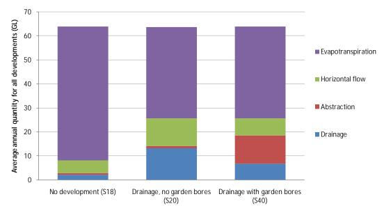
Figure 2.14 Water balance for the future medium climate scenario with no development, and development with drainage at ground level with and without garden bore extraction (source: Hall et al. 2010c)
