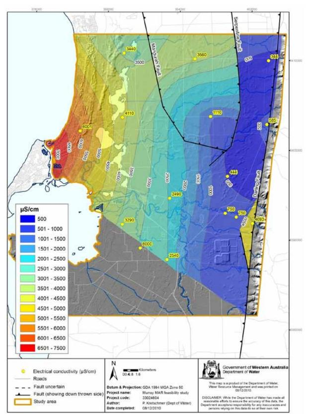
Figure 2.12 Cattamarra Aquifer electrical conductivity (temperature compensated to 25°C)
