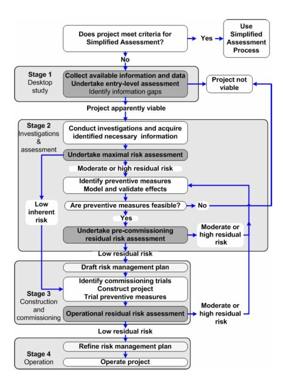
Figure 1.2 Stages of investigation for a managed aquifer recharge project (source: NRMMC 2009)
