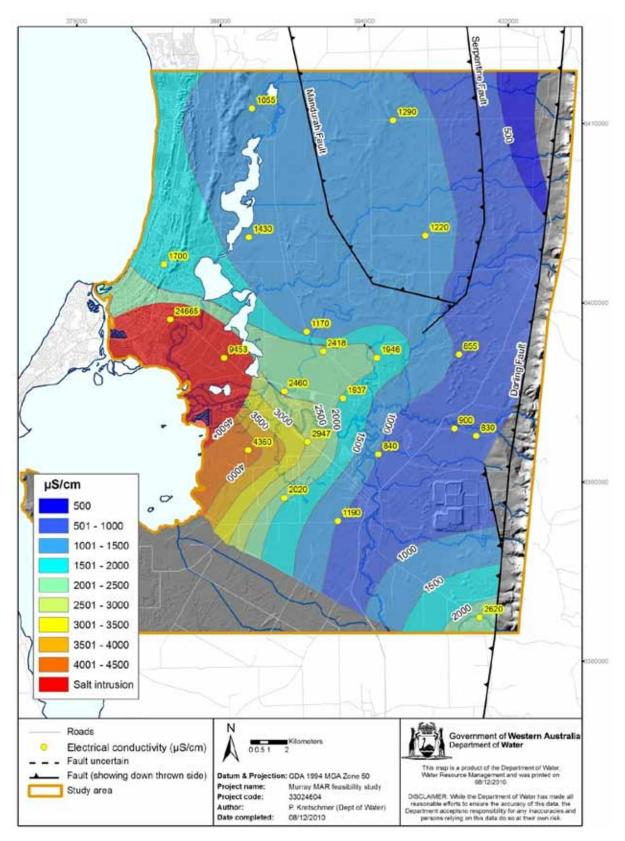
Figure 2.9 Combined lower Leederville Aquifer electrical conductivity (temperature compensated to 25°C)
