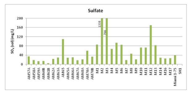
Chart B.7 Sulfate concentrations in groundwater within the Leederville Aquifer.
