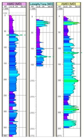
Figure A.11 Geophysical logs for AM62 (west), Yangedi Rd (centre), and AM63 (east). The Mandurah Fault is mapped between Yangedi Rd and AM62, with the formations on the east being downthrown relative to the units to the west. The green-clay marker bed is marked with the dashed green line.
