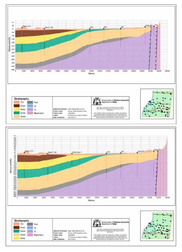
Figure 2.5 (top) and Figure 2.6 (bottom) Cross-sections of the revised geology interpretation
