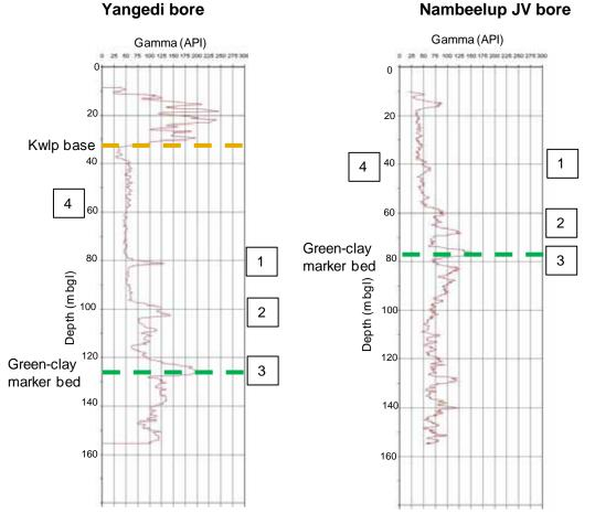
Figure A.9 Gamma and resistivity logs for Yangedi Rd and Nambeelup JV private bores. Note the overlying Pinjar Formation (Kwlp) in the Yangedi bore and the large gamma peak at the green-clay marker bed.
