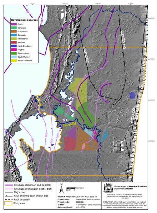
Figure A.1 Existing contours for South Perth Shale (Kws) base contours in m AHD
