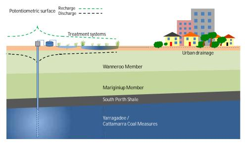
Figure 3.1 Conceptual diagram of an ASR scheme in the study area
