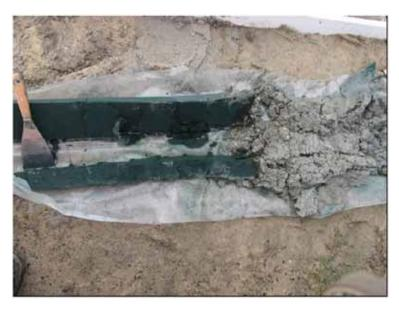
Figure A.7 Core from HS097 before being placed in the core tray. Note the abrupt transition from the Rockingham Sand to the green-clay marker bed at 67.5 mbgl. Photo courtesy Claire Johnsen, GHD
