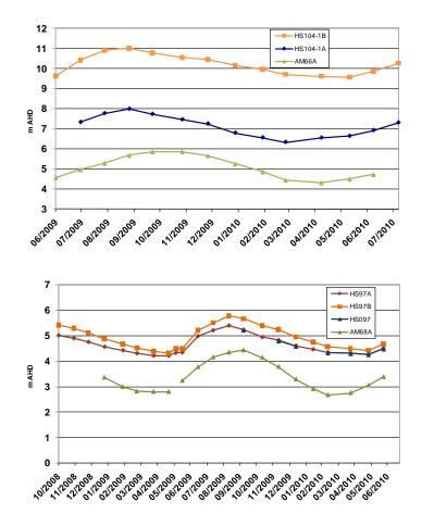
Chart 2.1 Hydrograph for the Superficial – Leederville Aquifer interaction. A) HS 104-B – Superficial Aquifer; HS104-1A – upper Leederville Aquifer; AM66A – lower Leederville Aquifer. B) HS97A; HS97B – Superficial Aquifer; HS097 – upper Leederville Aquifer; AM66
