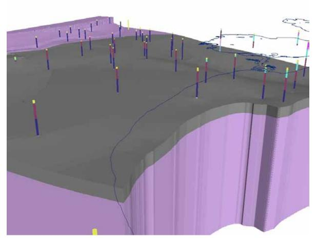
Figure A.3 An example of the surface for the South Perth Shale (grey) fitting through the picks in the bores. The South Perth Shale is pink in the bores (just visible at the base of some bores), the Mariginiup Member is marked dark blue, and the Wanneroo Member dark red. The underlying purple-coloured unit is the Cattamarra Coal Measures.
