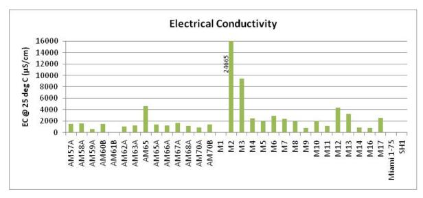
Chart B.1 Electrical conductivity values in groundwater within the Leederville Aquifer
