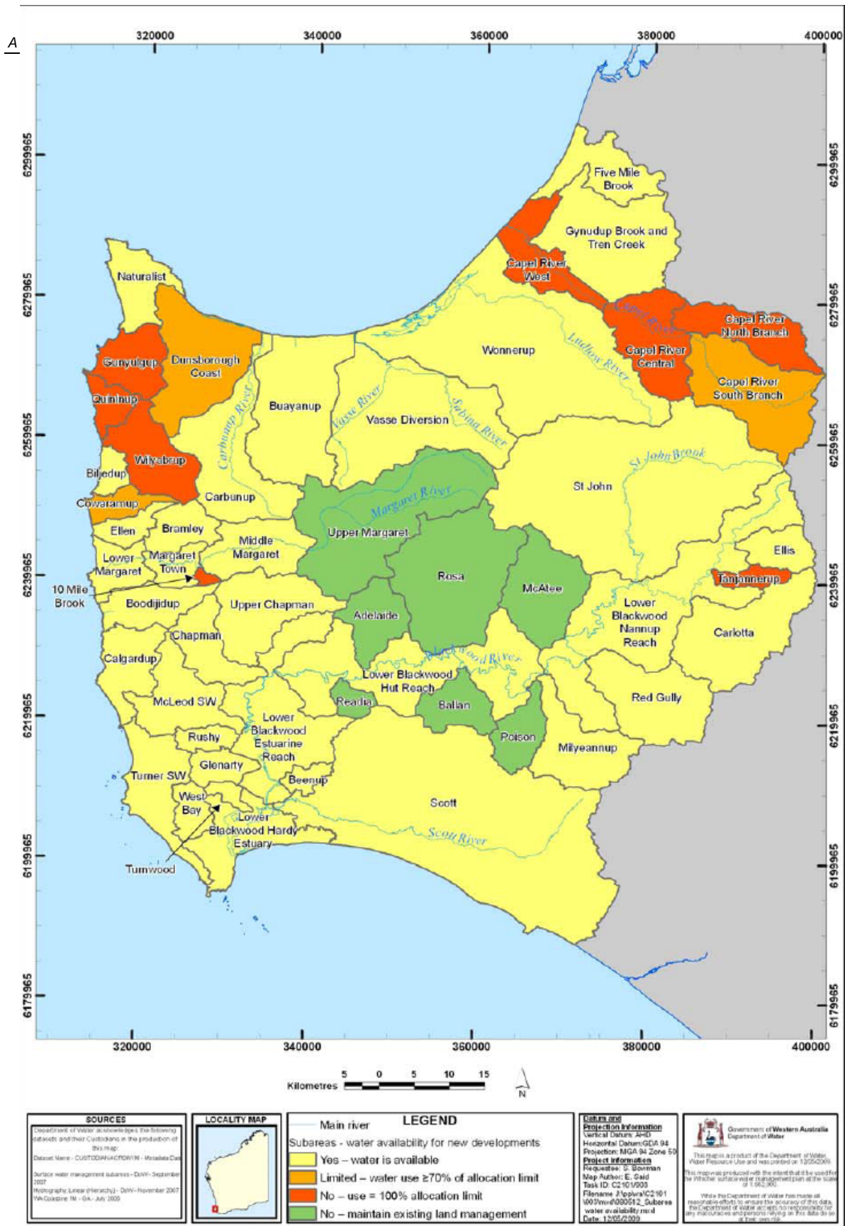
Figure 46: Surface-water availability in the Whicher area (DOW 2009).
