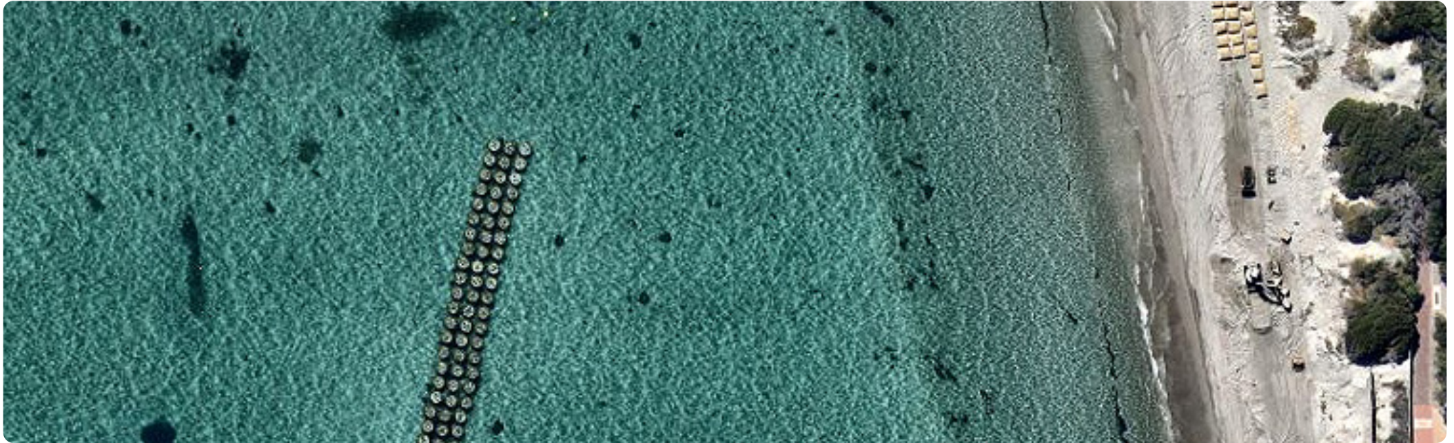
Engineered Fringing Reef installed near the CY O'Conner, designed to generate wave breaking and reduce coastal erosion. Source: Nearmap. Image taken April 2022.
