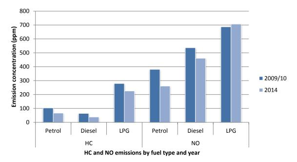
Figure 6. Emission averages by fuel type 2009–10 and 2014. Note: HC and NO measured as concentration in ppm
