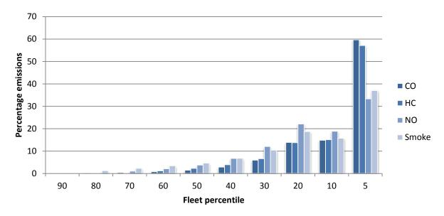
Figure 4. Fleet emissions by percentile range. The worst 5% of the fleet are responsible for 59% of CO, 57% of HC, 32% of NO and 36% of smoke (particulates)
