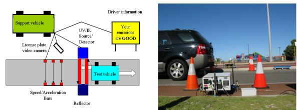
Figure 2: Schematic diagram of the RSD monitoring equipment<sup>1</sup> (left) and RSD source/detector and reflector in operation (right)
