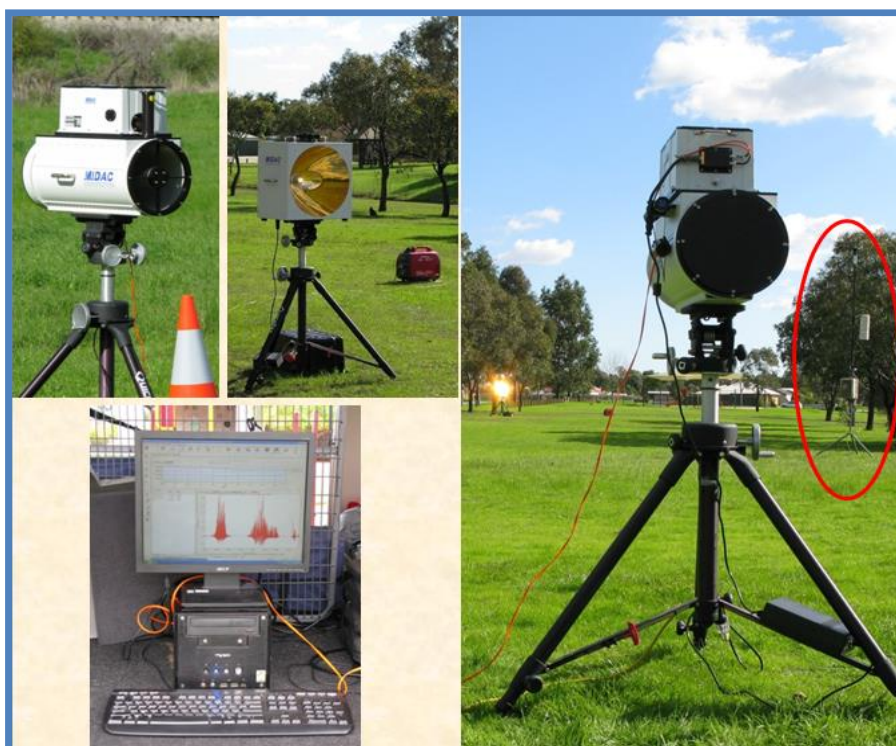
Figure 2.3.1 Typical OP-FTIR monitoring set-up. Images displayed clockwise from left are OP-FTIR detector, OP-FTIR light source, OP-FTIR detector and source separated by a 60-metre sample path with meteorological sensors on mast (circled in red) and computer logging measurements.
