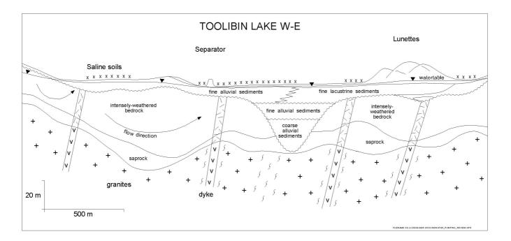
Figure 8. West-east hydrogeological cross-section of Toolibin Lake
