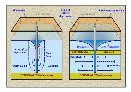
Figure 2. The responses of confined and unconfined aquifers to groundwater pumping (From ABC's of Groundwater, Centre for Groundwater Studies, 2000)
