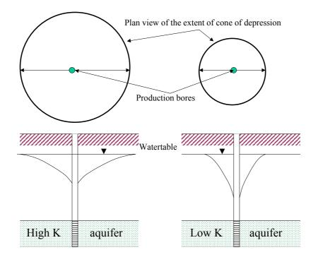
Figure 3. Drawdown cones for aquifers with high and low hydraulic conductivity (From ABC's of Groundwater, Centre for Groundwater Studies, 2000)
