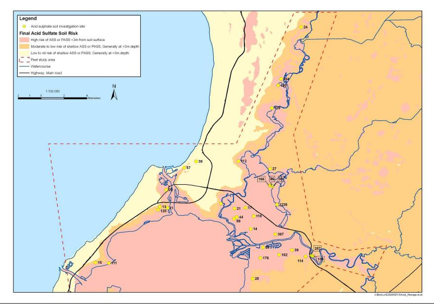
superficial sediments around the Peel Inlet, Serpentine River and Murray River. Note: map not displayed to scale.
