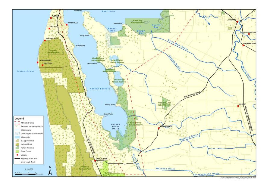
Figure 3: Initial ASS risk map (based on 1:50 000 scale environmental and urban geology mapping) and superficial formation investigation sites (Peel inlet, Serpentine and Murray Rivers). Note: map not printed to scale.
