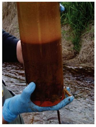
*Figure 24* Surficial sediments within the drain (site 6100095) showing the presence of iron floc.
