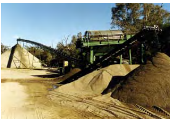
Screening plant which receives sand from the Burlong dredge (Photo courtesy Bernard Kelly)
