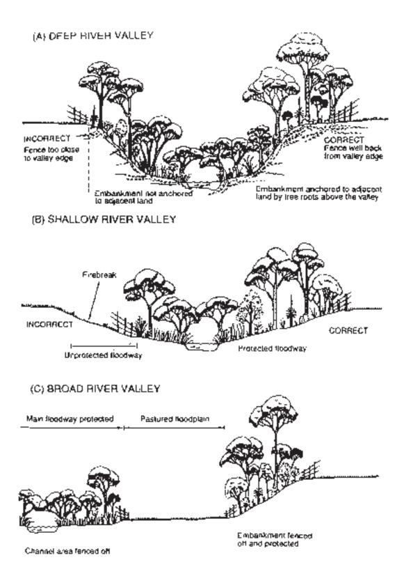
Figure 4: Placement of fences in relation to the river valley (after WRC, 2000c)
