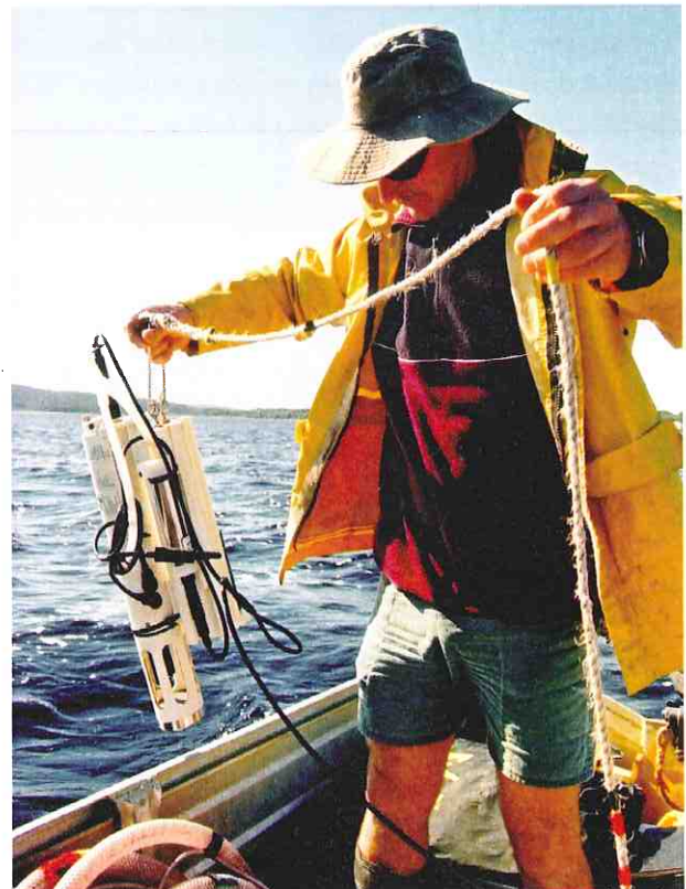
The hydro-lab used for the collection of data for the monitoring of the Inlet (photo Catherine MacCallum)
