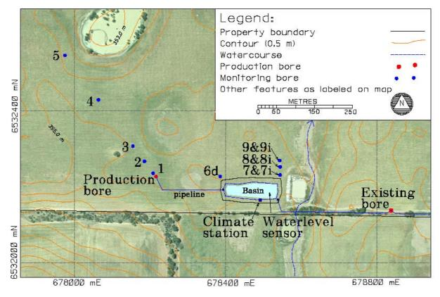
Figure 8 Layout of project site at Bodallin
