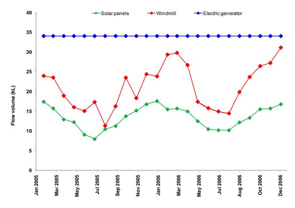
Figure 20 Simulated average daily discharge for each month of 2005 and 2006 for solar, wind and generator powered pumping
