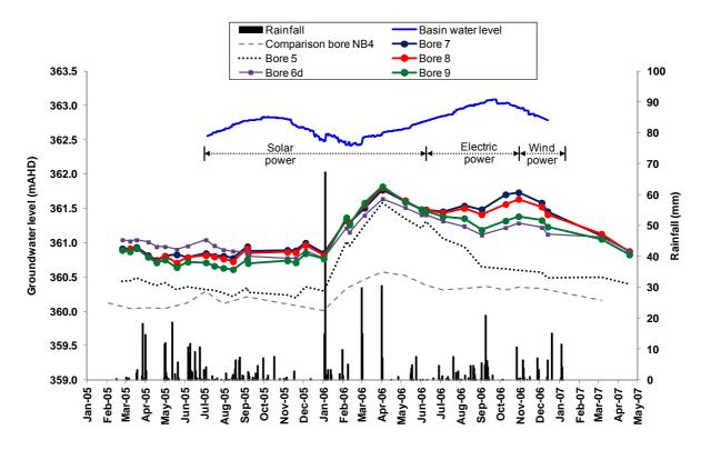
Figure 13 Groundwater levels in basin bores 7–9 compared to bore 5 and comparison bore
