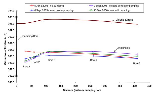
Figure 11 Watertable profiles of transect bores 1–5 during solar, electric and wind powered pumping
