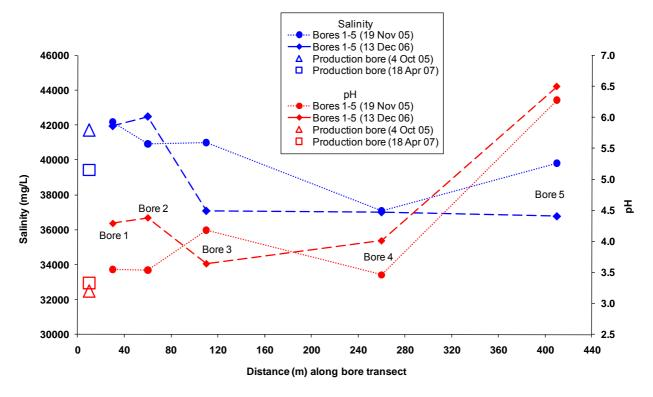
*Figure 12 Groundwater quality profiles for production bore and transect bores 1–5*
