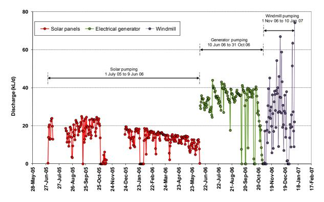
Figure 17 Pumping rates produced by solar, generator, and wind power
