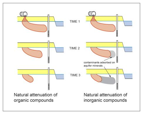
Figure 3: Shrinking of groundwater contamination plumes because of natural attenuation processes for organic (destructive, irreversible NA processes) and inorganic contaminants (generally non-destructive, reversible NA processes).
