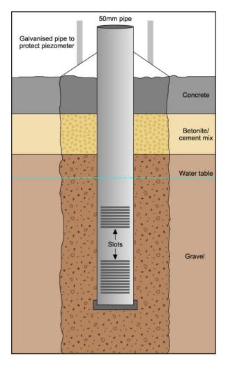
Figure 5: Typical construction of a groundwater monitoring bore (Sundaram et al., 2009)
