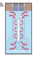
Figure 7: Sampling problems associated with the use of (a) high flow rate pumps and (b) bailers or inertial pumps with a foot-valve ('jiggle' pumps).
