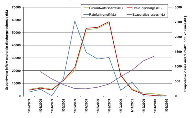
Figure 25 In-channel water balance for downstream drain between Stations B and C
