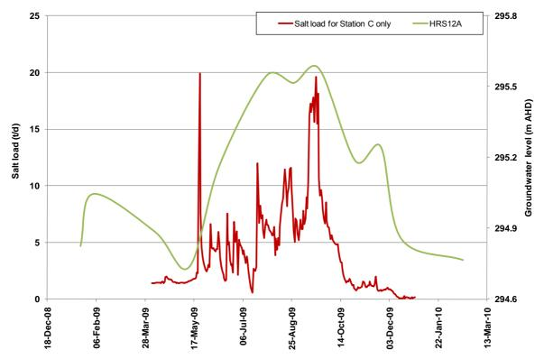
Figure 29 Comparison bore groundwater levels versus salt loads
