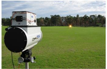
FTIR setup—light source in the distance aligned with the detector
