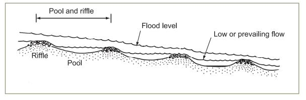
Figure 7 A series of rock riffles in a waterway
