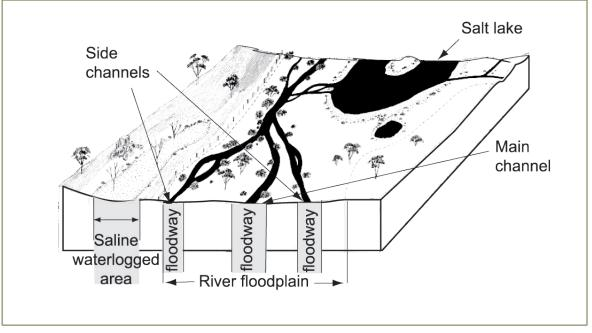
Figure 2 Cross-section of a typical watercourse in the Avon catchment (WRC, 2003)
