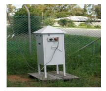
**Figure 3:** A high volume sampler used to monitor particulates and heavy metals
