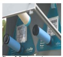
Figure 2: Passive samplers
