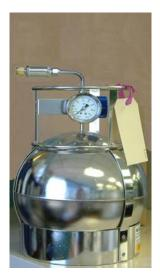
Figure 4: A stainless steel sampling canister used in the community sampling program
