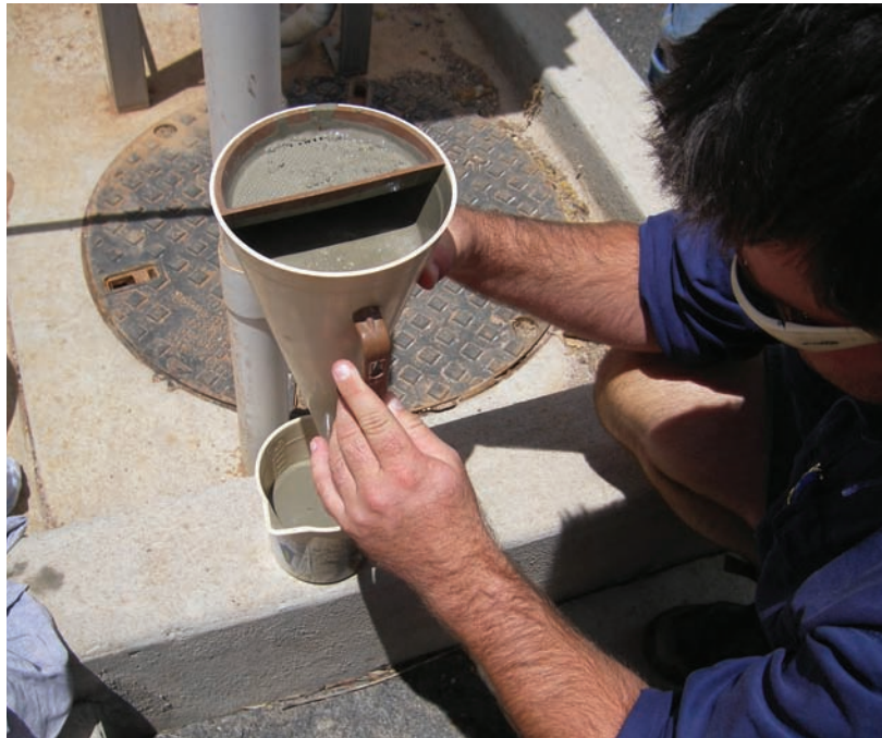
Measuring viscosity using a Marsh funnel
