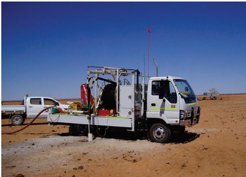
Mobile pump test unit (small flow)
