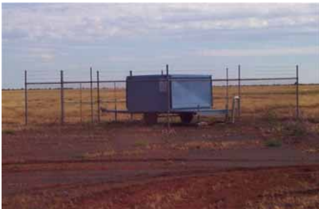
Figure 3.11 Karratha MS - Doppler acoustic sounder.
