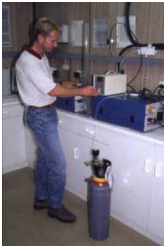
Figure A1 A DEP staff member performing a monthly calibration at the Dampier air quality monitoring station.
