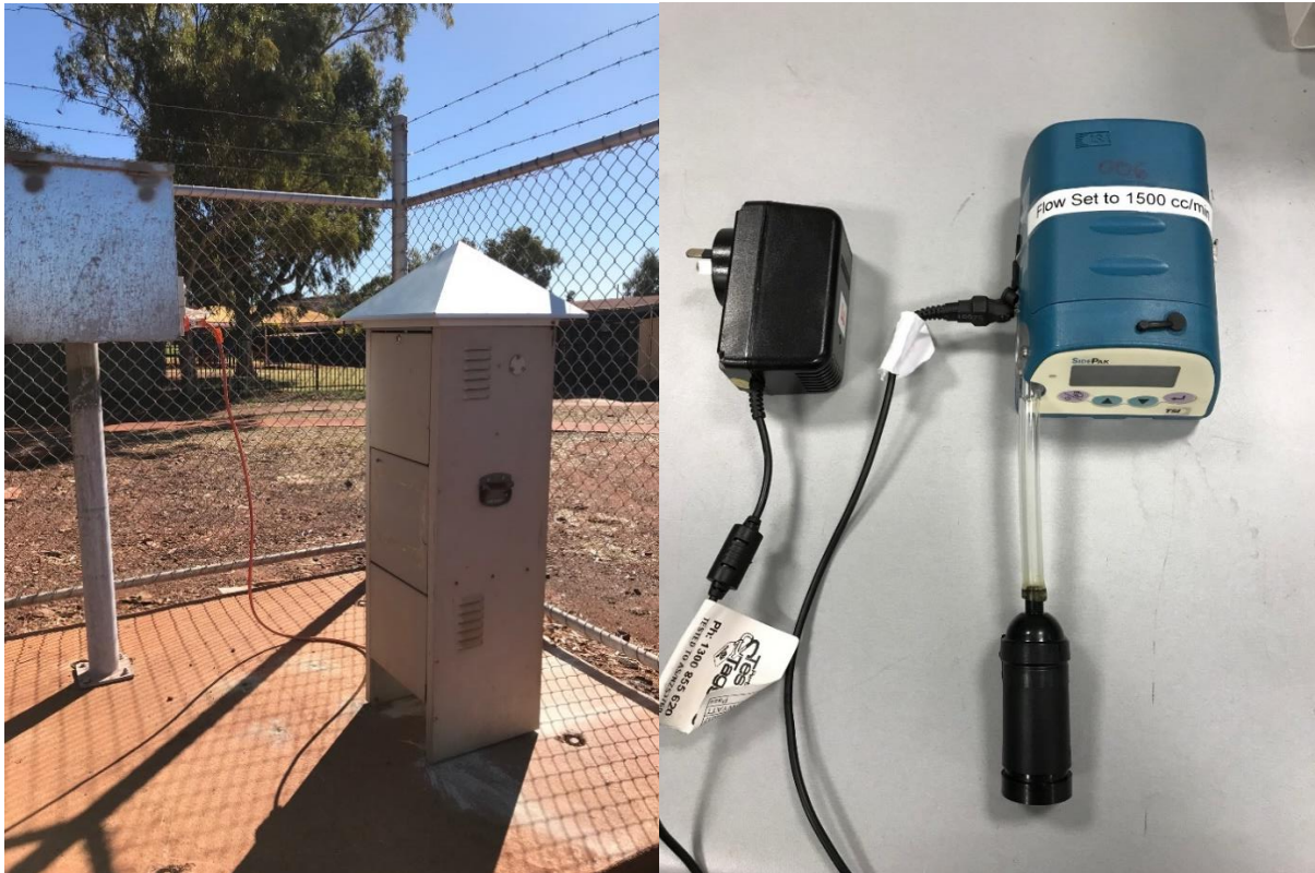
Figure 4: High volume air sampler (left) and asbestos sampling equipment (right).
