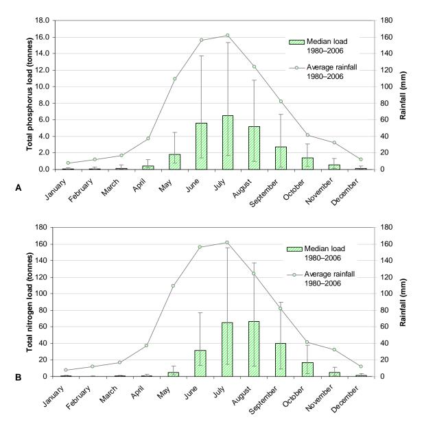
*Figure 7.10.* The breakdown of modelled monthly phosphorus loads (A) and monthly nitrogen loads (b) for the period 1980–2006. The error bars denote 25th and 75th percentiles, and average monthly rainfall is for the Geographe catchment.
