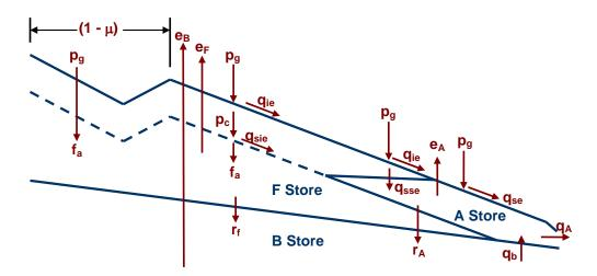
Figure 2.2. Schematic of a hill-slope cross-section assumed in SQUARE, and the definition of the subsurface water stores (Viney & Sivapalan 2001).
