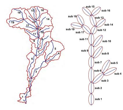
*Figure 2.1.* Subcatchment organisation (i.e. surface connection) based on a river network of 19 subcatchments.
