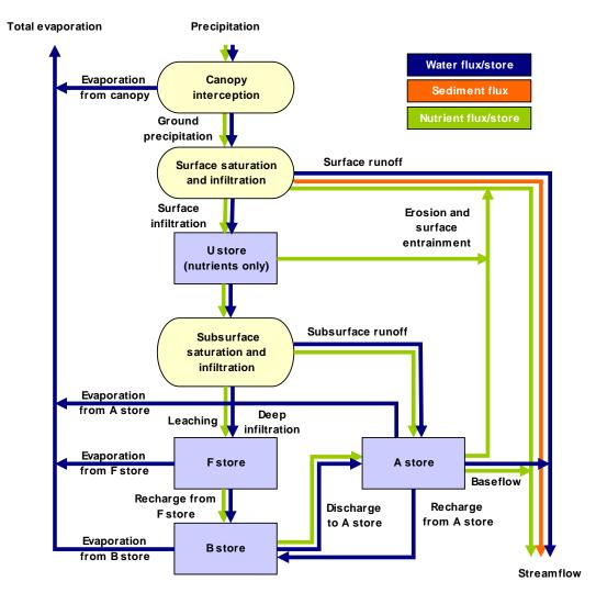
Figure 2.3. Small catchment model (building block model) in SQUARE for water, sediments and nutrients (Zammit et al. 2005).
