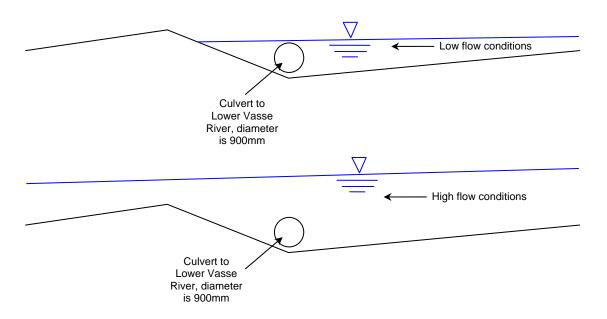
*Figure 7.16.* Conceptual cross-section of the Vasse Diversion Drain displaying the position of the culvert to the Lower Vasse River.
