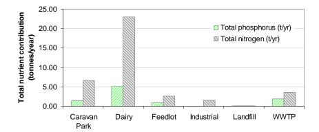
Figure 7.5. Nutrient-load contributions from various point-source components.
