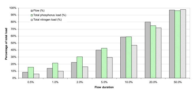
*Figure 7.12. Modelled cumulative flow and nutrient-load percentages for various duration periods.*
