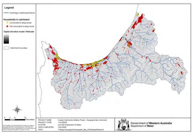
Figure 3.10. Infill sewerage and septic-tank locations (2005).
