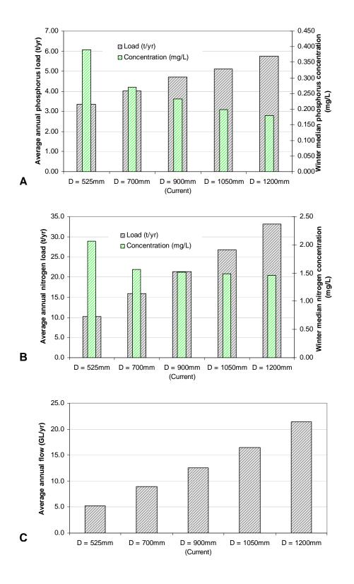
*Figure 7.17.* The effects of changing culvert diameter sizes on the load and winter median concentration for phosphorus (A), nitrogen (B) of the outflow (C) from the Lower Vasse River.
