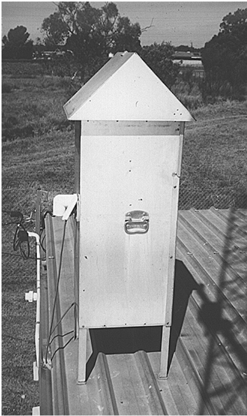
Figure 5.9 - High volume sampler with a TSP head.
