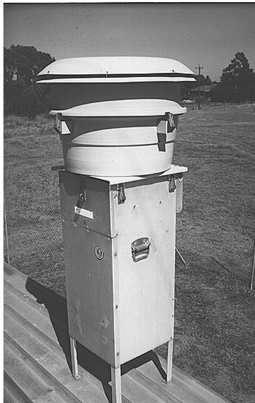
Figure 5.10 - High volume sampler with PM10 head.
