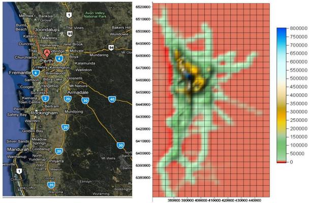
Figure 7: The spatial distribution of the estimated particulate matter (gram/day) for the Perth Airshed from on-road vehicles based on 2011/2012 emissions modelling
