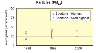
Figure 4.8 Summary of  $PM_{2.5}$  data measured by a TEOM at the Boodarie monitoring station, showing the highest and sixth highest 24-hour average concentration each year.
