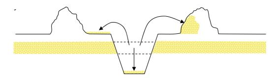
Figure 17 A schematic cross-section showing options for placing excavated alkaline subsoils for use in drain spoil, to enhance alkalinity in runoff from berms or directly in drain base
