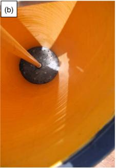
Figure 43 The up-flow tank reactor (a) after assembly of the column and the support tower (with the 50 mm diameter polythene inflow through the top and outflow via the 90 mm PVC)and (b) a view of the diffuser plate inside the reactor after installation
