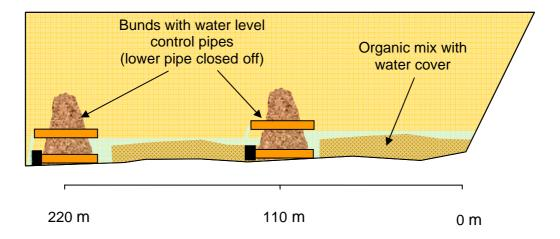
Figure 22 Cross-sectional view of bunding and water-level control pipe layout in the 200 m in-drain composting bed at Wallatin Creek. Note water level adjusted to achieve water cover over organic matter laid on uneven drain base.
