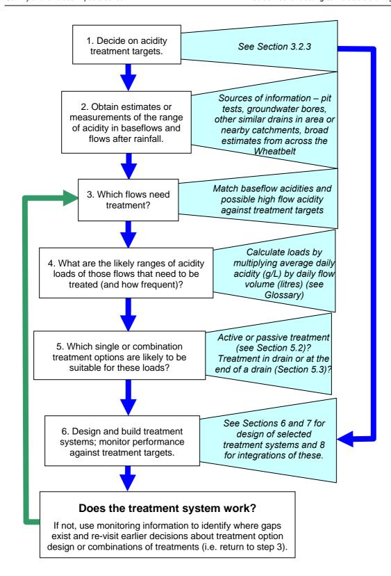
Figure 9 Key steps in making decisions that help in the design (including where information can be obtained) and adaptive management of treatment systems
