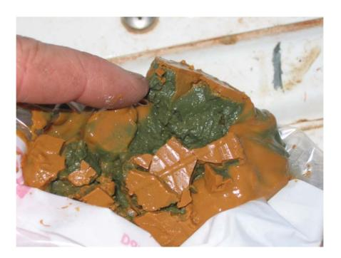
Figure 49 Iron- and aluminium-rich sludge from the settling tanks of the hydrated lime dosing unit. The green is due to ferrous hydroxide which oxidises to orange iron oxide on exposure to air.
