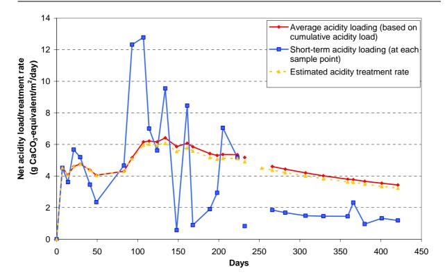
Figure 38 Average acidity loading, estimated treatment rates (correcting for estimated untreated acidity in outflows) and short-term variations in net acidity loading for the pilot composting wetland at Beacon. Absence of points and breaks in plotted lines indicate when inflow was shut down or there was no outflow.
