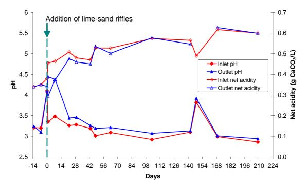
Figure 14 Net acidity and pH in inflow and outflow water of a 210-m drain section treated with limesand
