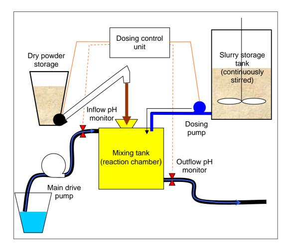
Figure 47 Elements of a hydrated lime dosing unit (with slurry dosing or dry power addition)
