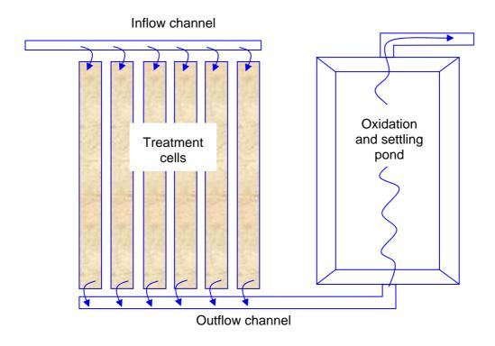
Figure 31 Outline plan diagram of a simple treatment wetland with a series of linear treatment cells and outflow to an oxidation and settling pond prior to discharge
