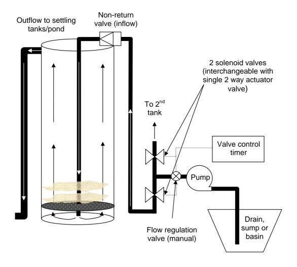
Figure 39 Conceptual schematic of a pulsed up-flow lime-sand reactor
