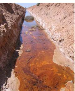
Figure 15 Iron oxide crust formation on lime-sand implicated in slowing neutralisation rates
