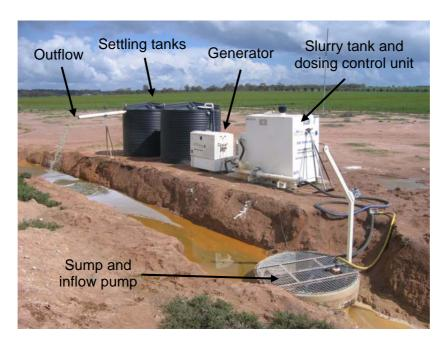
Figure 48 The hydrated lime dosing unit treating water at the end of the Wallatin Creek drain
