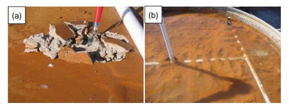
Figure 45 Iron crusting (a) formed after several days on the surface of the lime-sand and (b) gradually reduced the infiltration of water through the sand and caused water to pond to 10 cm depth
