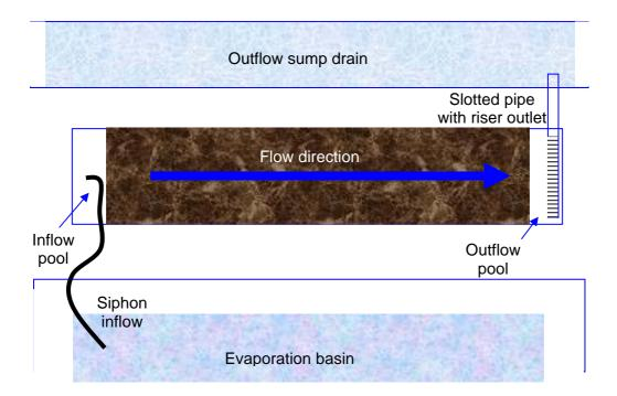
Figure 34 Plan view diagram for the pilot composting wetland constructed at Beacon
