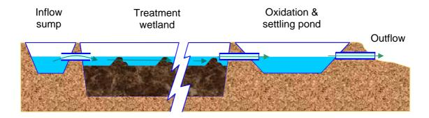
Figure 33 Conceptual layout of composting treatment wetland with inflow sump and polishing oxidation/settling pond
