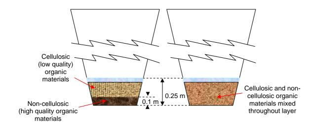
Figure 21 Cross-section views of examples of vertical placement arrangements of organic materials in composting bed design
