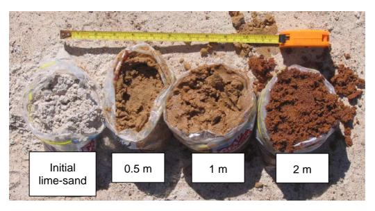
Figure 46 Iron armouring of lime-sand sampled at a range of depths (below outflow) from a pulsed upflow reactor, evident as red staining after neutralising 580 kL acidic water over 8 days
