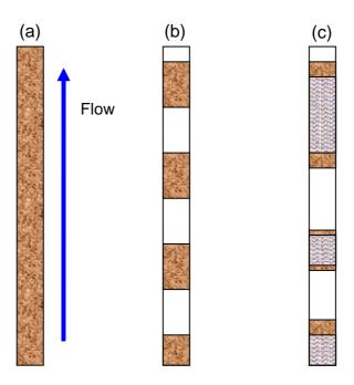
Figure 20 Plan views of organic material placement along drains in composting bed design: (a) full drain length, (b) regularly spaced sections and (c) concentrated and aligned with ponds (blue waves) selected after drain construction
