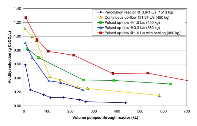
Figure 44 Efficiency of acidity treatment (reduction of outflow acidity compared with inflow acidity)
