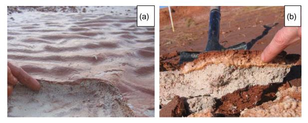
Figure 30 Thin mud layer (<5 mm) covering lime-sand after the first batch (a) and the mud and salt crust layer (up to 20 mm deep) covering the lime-sand after Batch 3
