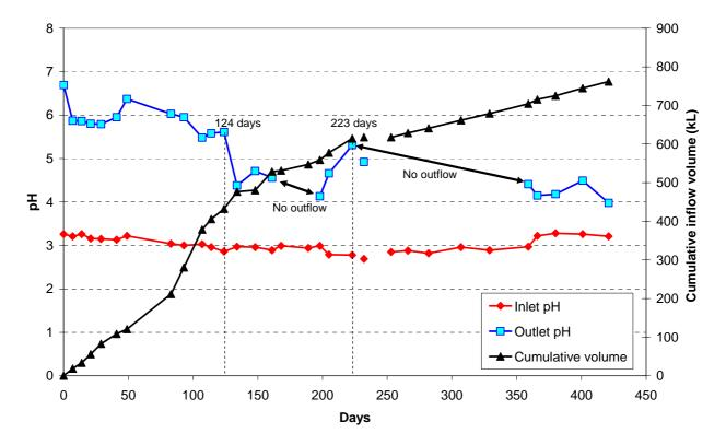
Figure 36 Inflow and outflow pH and cumulative inflow volume for the pilot composting wetland at Beacon. The absence of data points and breaks in plotted lines indicate when inflow was shutdown or there was no outflow.
