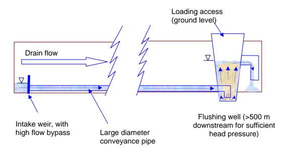
Figure 26 Schematic cross-section of a diversion well illustrating intake and downstream well outlet within a drain
