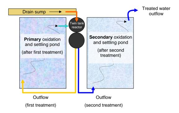
Figure 40 Schematic diagram of a two-staged treatment system using a single twin-tank lime-sand tank reactor with water initially pumped from the drain sump into the primary pond and treated a second time with discharge to the secondary pond.
