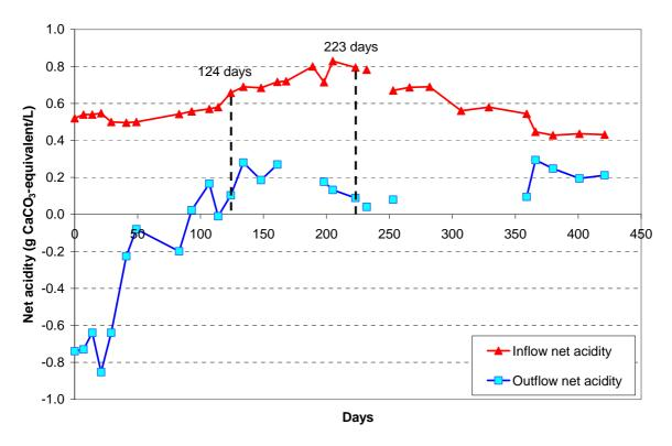
Figure 37 Inflow and outflow net acidity for the pilot composting wetland at Beacon. The absence of data points and breaks in plotted lines indicate when inflow was shut down or there was no outflow. Instances when outflow water containing alkalinity as bicarbonate are reported as negative net acidity values.
