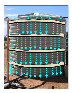
Figure 42 Flow path through four tables on which lime-sand was suspended in the percolation tank reactor
