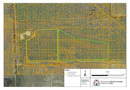
Figure 6 Boundary of project plots, 10 cm contours and flow directions Data source: Westclay Pty Ltd
