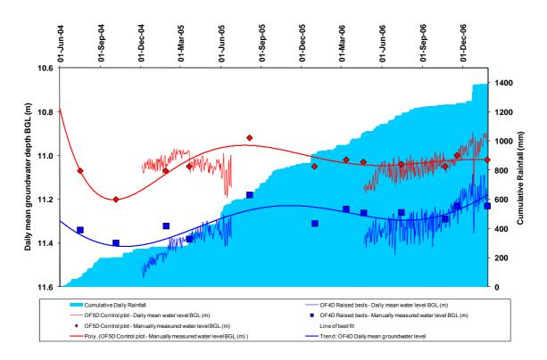
Figure 27 Comparison of groundwater levels in bores OF4D (raised bed) and OF5D (control bed)
