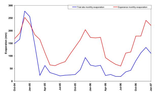
Figure 14 Total monthly evaporation at trial site gauging station and Esperance station, August 2004– January 2007
