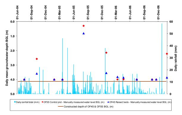
Figure 25 Comparison of manually measured groundwater levels in bores OF4S (raised bed) and OF5S (control bed)
