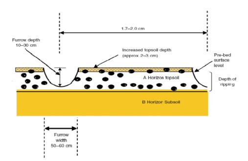
Figure 2 Schematic diagram of a raised bed
