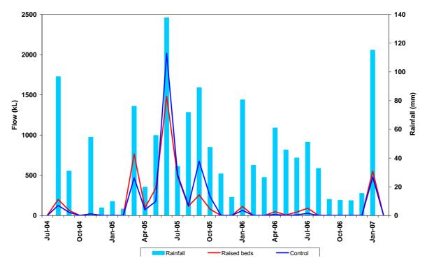
Figure 16 Comparison of total monthly surface water flow (kL) of raised and control beds with rainfall
