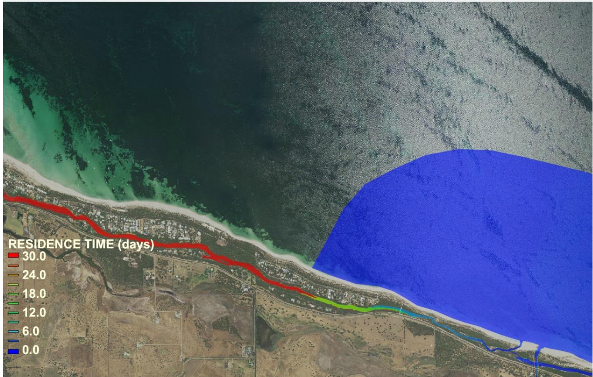
Toby Inlet closed, Station Gully open, culvert removed
