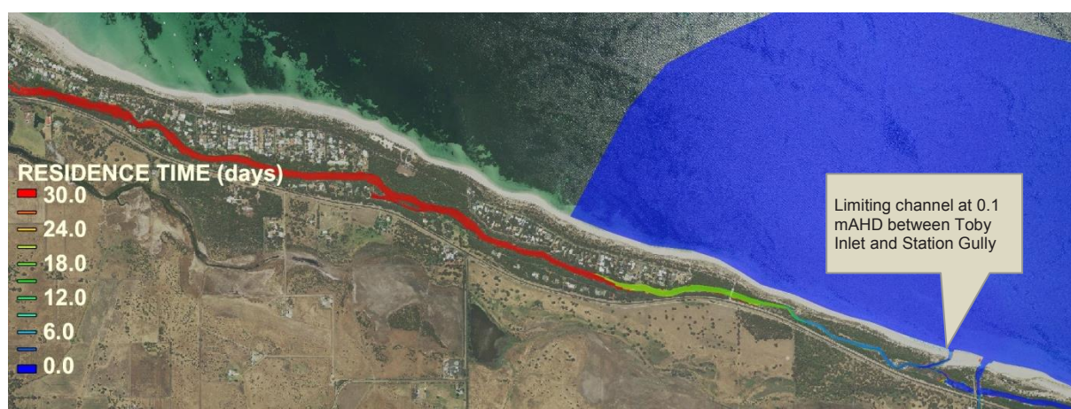
Figure 13 Residence time for Toby Inlet in January, Scenario 3 (single opening at Station Gully)
