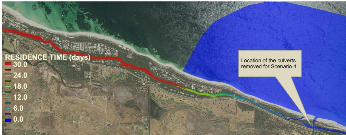
Figure 15 Residence time for Toby Inlet in January, Scenario 4 (culvert removed)
