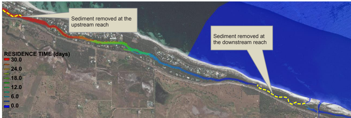
Figure 21 Residence time for Toby Inlet in January, Scenario 9 (sediment removal)
