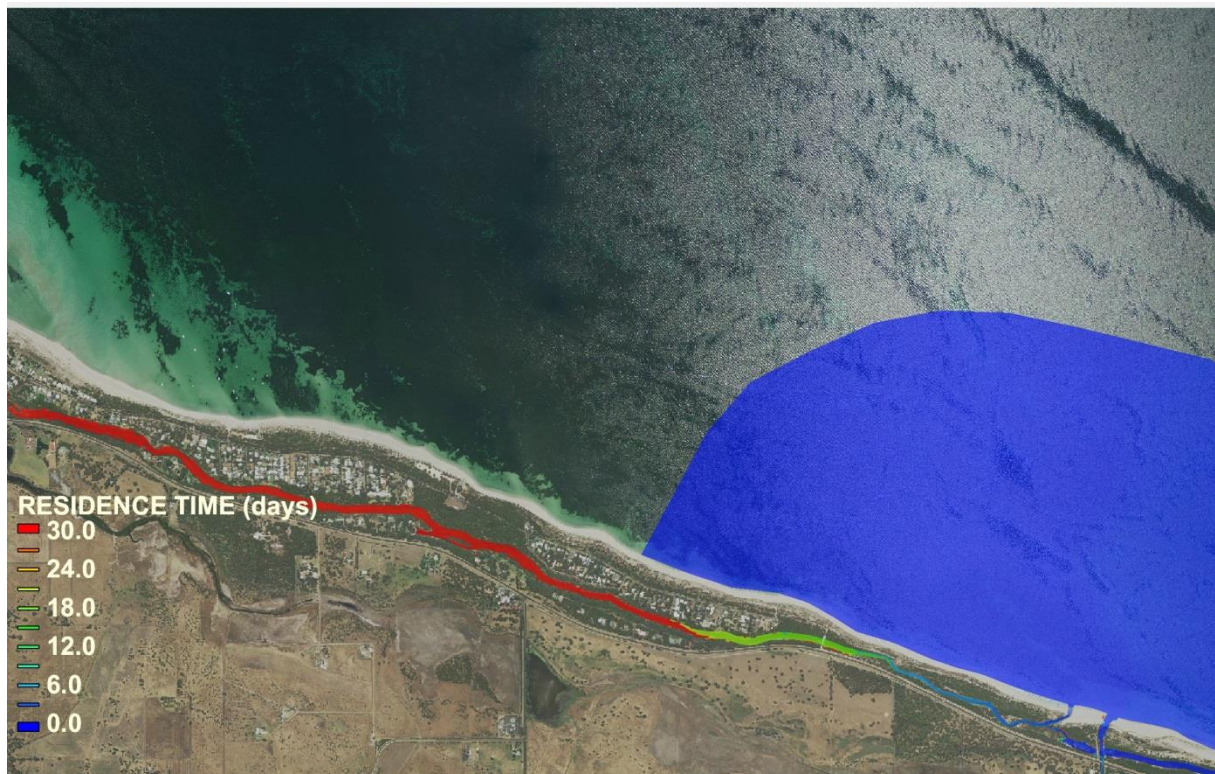
Toby Inlet closed, Station Gully open, increased to four culverts open
