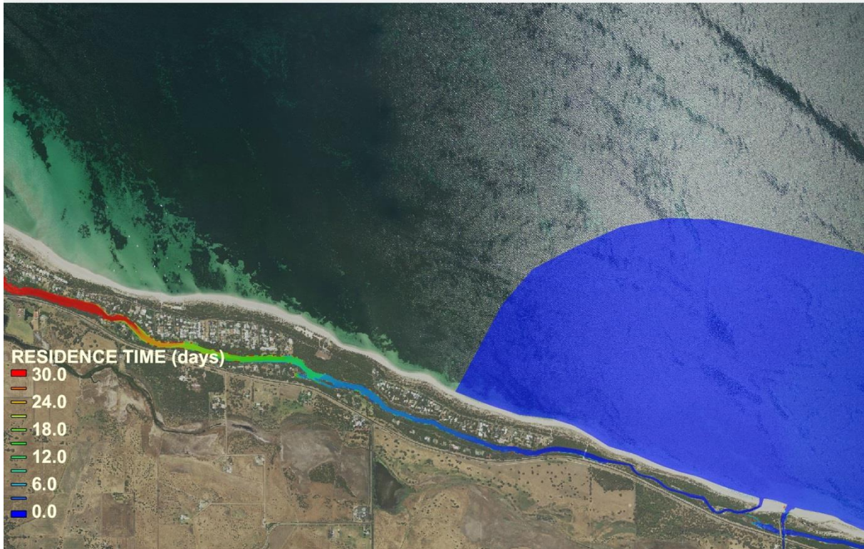
Toby Inlet open, Station Gully open, culvert open, lower section dredged to -0.5 mAHD
