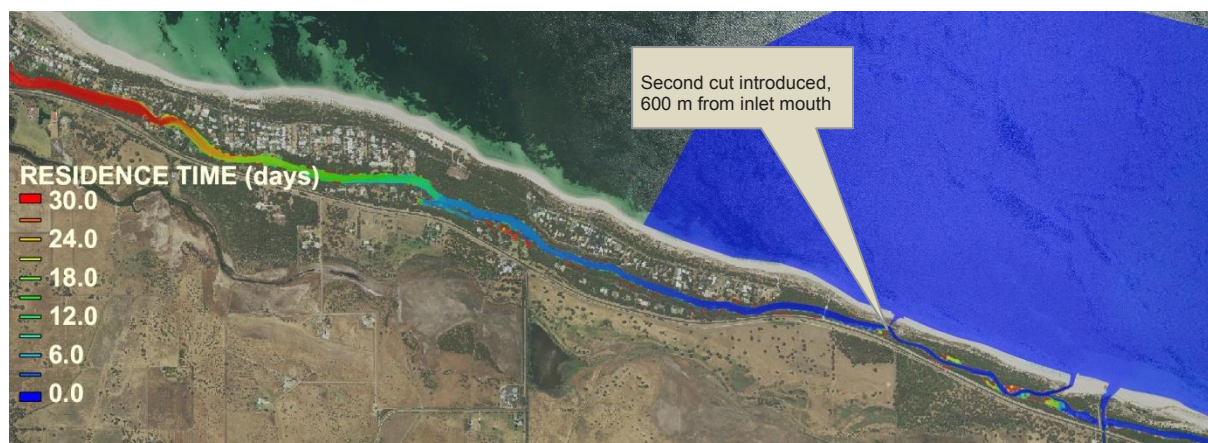
Figure 19 Residence time for Toby Inlet in January, Scenario 6 (introduction of a second cut)
