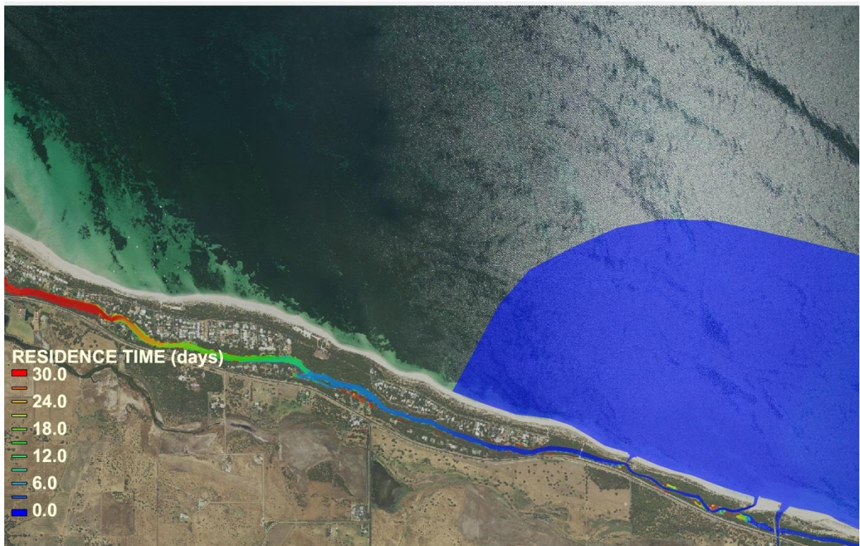
Toby Inlet closed, Station Gully open, culvert open, extra cut
