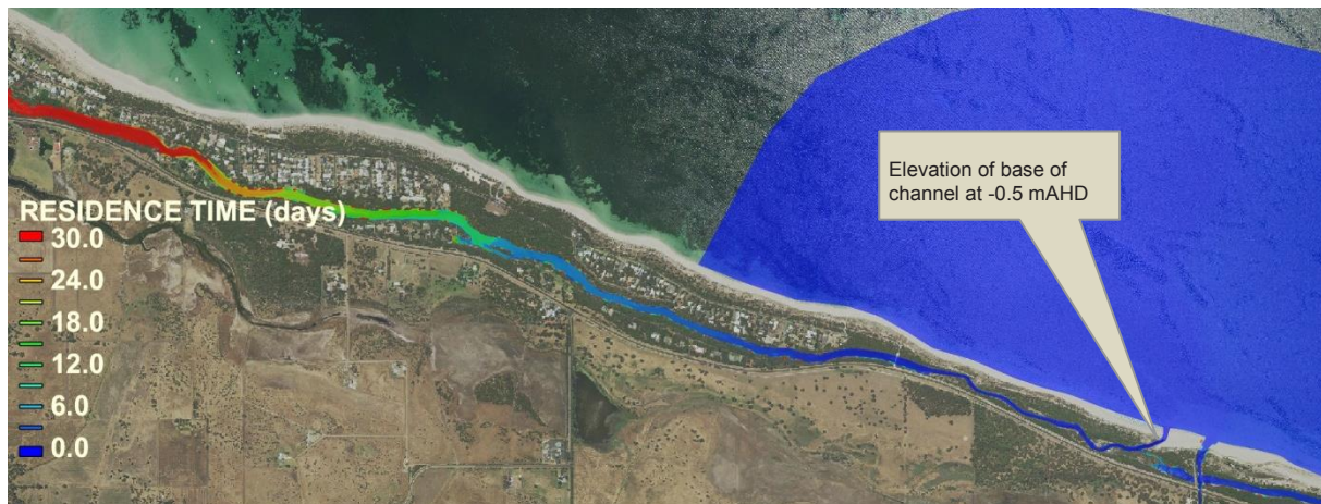
Figure 17 Residence time for Toby Inlet in January, Scenario 5 (mouth and sill excavated to -0.5 mAHD)
