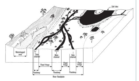
Figure 2. Cross sectional representation of a typical watercourse in the Avon catchment.
