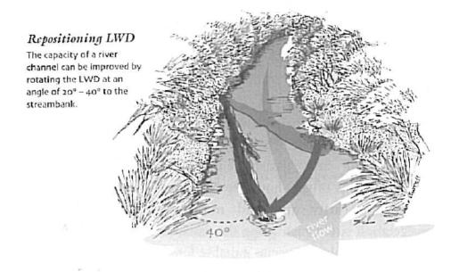
Figure 15: Repositioning large woody debris (Gippel et al. 1998)
