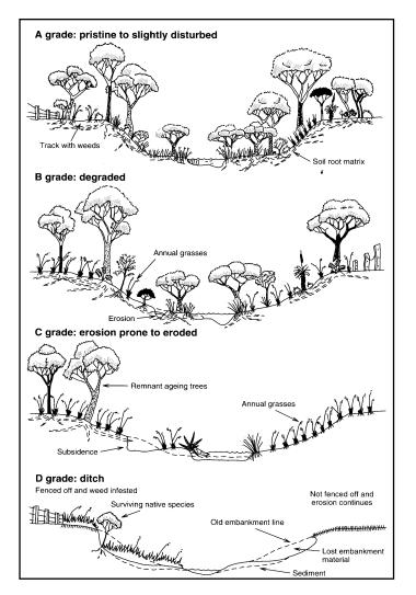
Figure 6: The four grades of river foreshore condition (A) pristine to (D) ditch (after Pen and Scott 1995)
