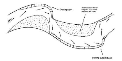
Figure 12: Outside bend bank erosion Arrows mark the direction of flow showing that outside bends have the greatest erosion potential, so the meanders migrate downstream (Raine and Gardiner 1995)
