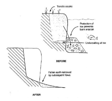
Figure 13: The use structural works to prevent undercutting (adapted from Raine and Gardiner 1995)
