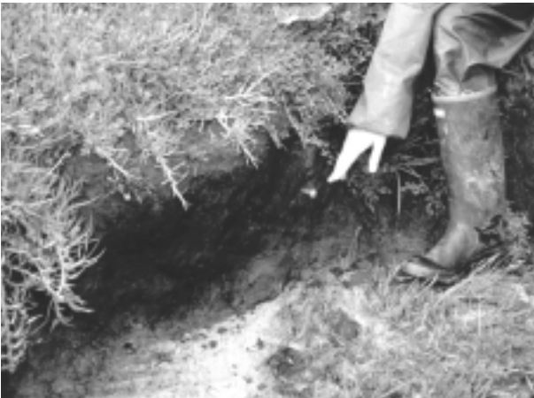
Figure 7. Shows an erosion pin in a creek bank. More of the pin is exposed as the bank surface erodes away.
