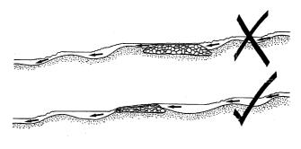
Figure 6: Riffle located on high point of channel profile.
