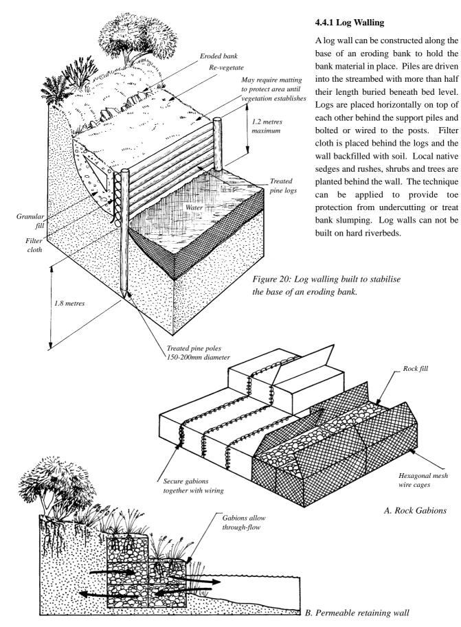
Figure 21: Stabilisation of steep banks using rock gabions.
