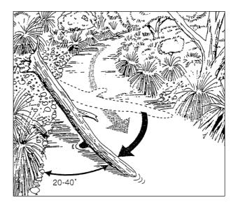
Figure 14: Large woody debris bank protection.
