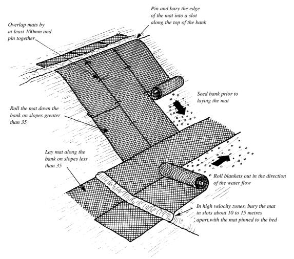
Figure 19: Installation of matting to prevent soil loss.
