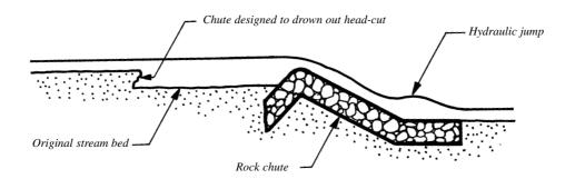
C. Chute designed to back-flood head-cut
