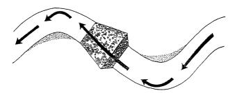
Figure 5: Riffle located at meander crossover.
