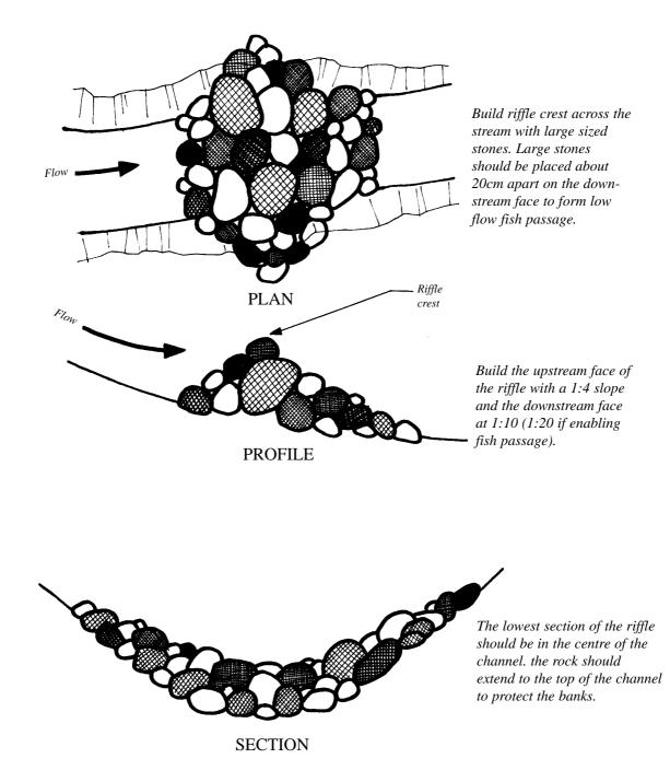
Figure 7: Schematic diagram for riffle construction.
