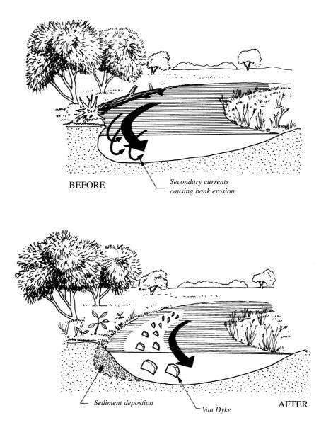
Figure 16: Vane dykes applied to reduce bank erosion.
