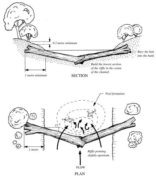
Figure 8: Log riffle cross-section and plan view.
