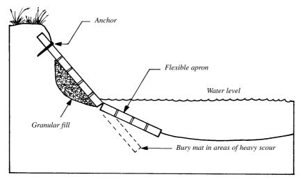
B. Concrete flexmat used for bank stabilisation
