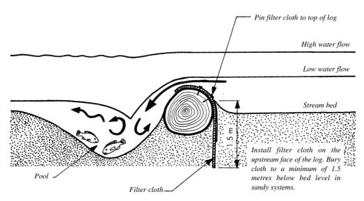
Figure 9: Installation of filter cloth on log riffle.
