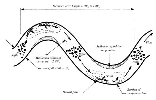
Figure 3: Meandering stream channel form.
