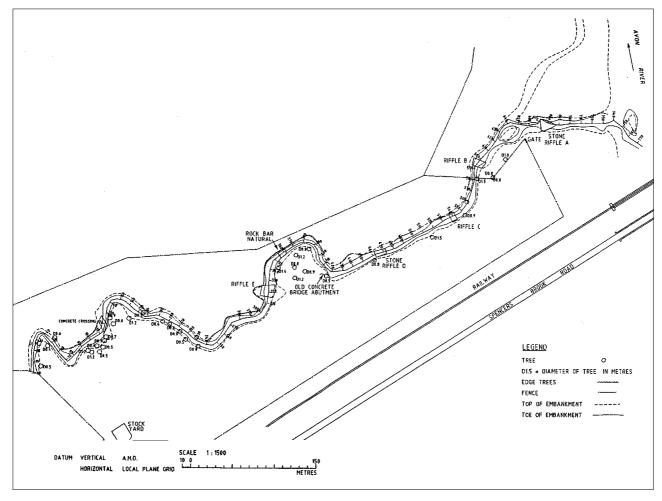
Figure 4: Spencers plan view of riffle sequence.
