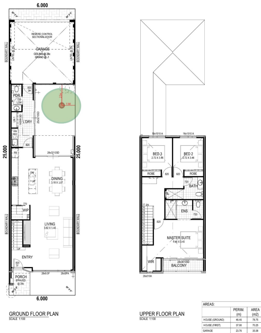
Figure 8 Example of Floor Plan which may be accommodated of R60 Laneway Lot
