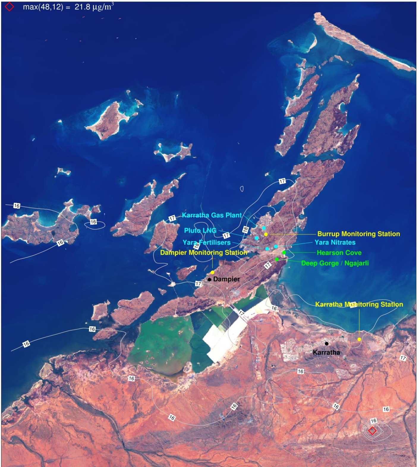
Figure 6-38. \text{PM}_{2.5} ( \mu\text{g}/\text{m}^3 ) annual max 24-hour concentrations for Scenario 2 (S2) for a subset of the CAMx 1.33 km domain centred over the Burrup Peninsula.
