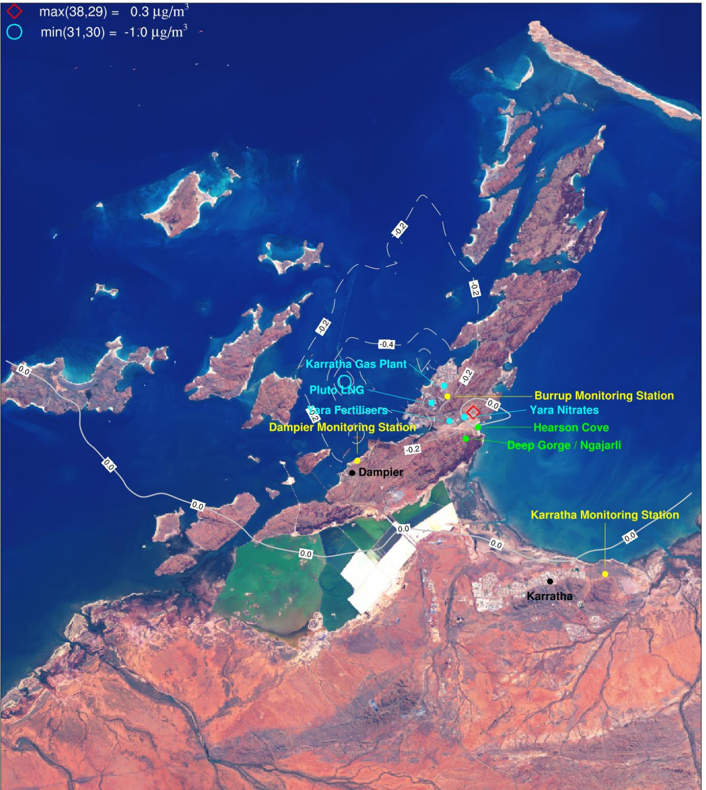
Figure 6-79. \text{PM}_{2.5} ( \mu\text{g}/\text{m}^3 ) change in annual average ground level concentrations from Scenario 2 due to future industry (S3-S2) for a subset of the CAMx 1.33 km domain centred over the Burrup Peninsula.
