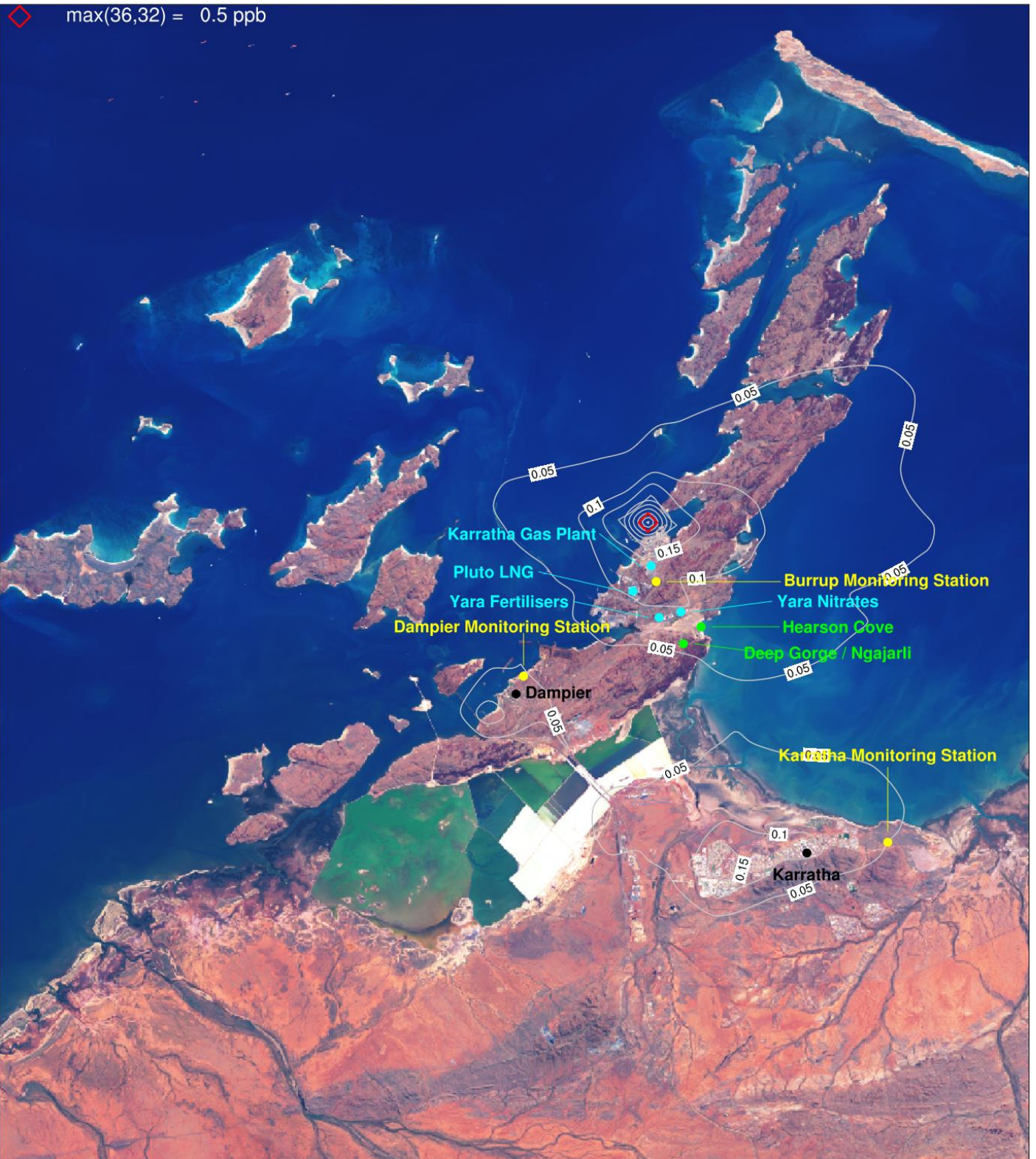
Figure 6-23. XYL (ppb) annual average concentrations for Scenario 2 (S2) for a subset of the CAMx 1.33 km domain centred over the Burrup Peninsula.
