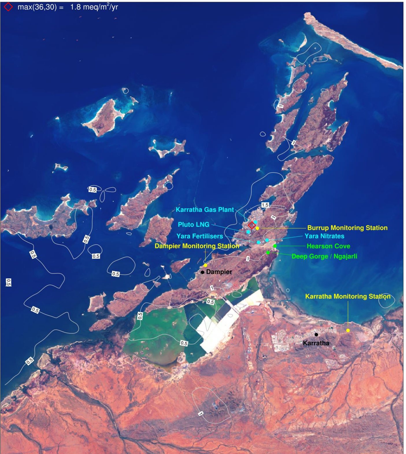
Figure 6-91. Annual total \text{PSO}_4 (sulphate; units: \text{meq/m}^2/\text{yr} ) deposition for Scenario 2 (S2) for a subset of the CAMx 1.33 km domain centred over the Burrup Peninsula.
