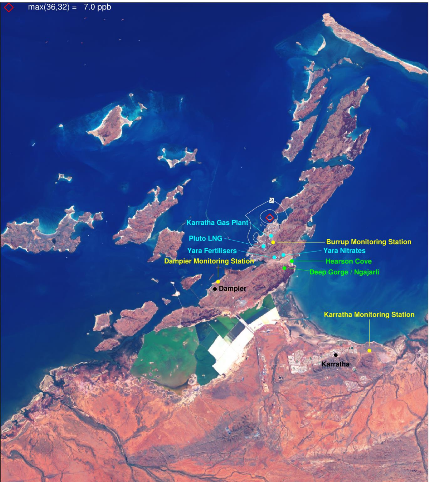
Figure 6-45. XYL (ppb) annual max 24-hour ground level concentrations due to industry (S2-S1) for a subset of the CAMx 1.33 km domain centred over the Burrup Peninsula.
