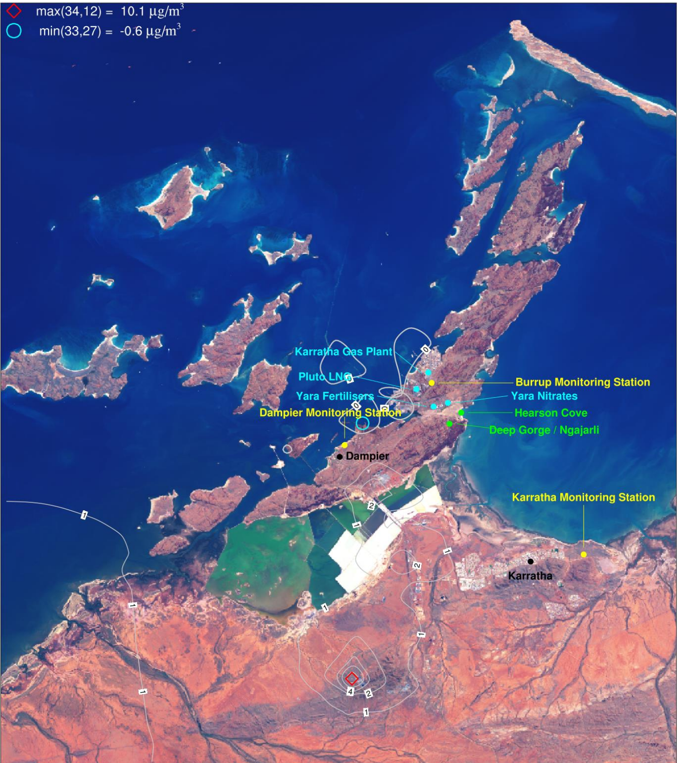
Figure 6-77. \text{PM}_{10} ( \mu\text{g}/\text{m}^3 ) change in annual average ground level concentrations from Scenario 2 due to future industry (S3-S2) for a subset of the CAMx 1.33 km domain centred over the Burrup Peninsula.
