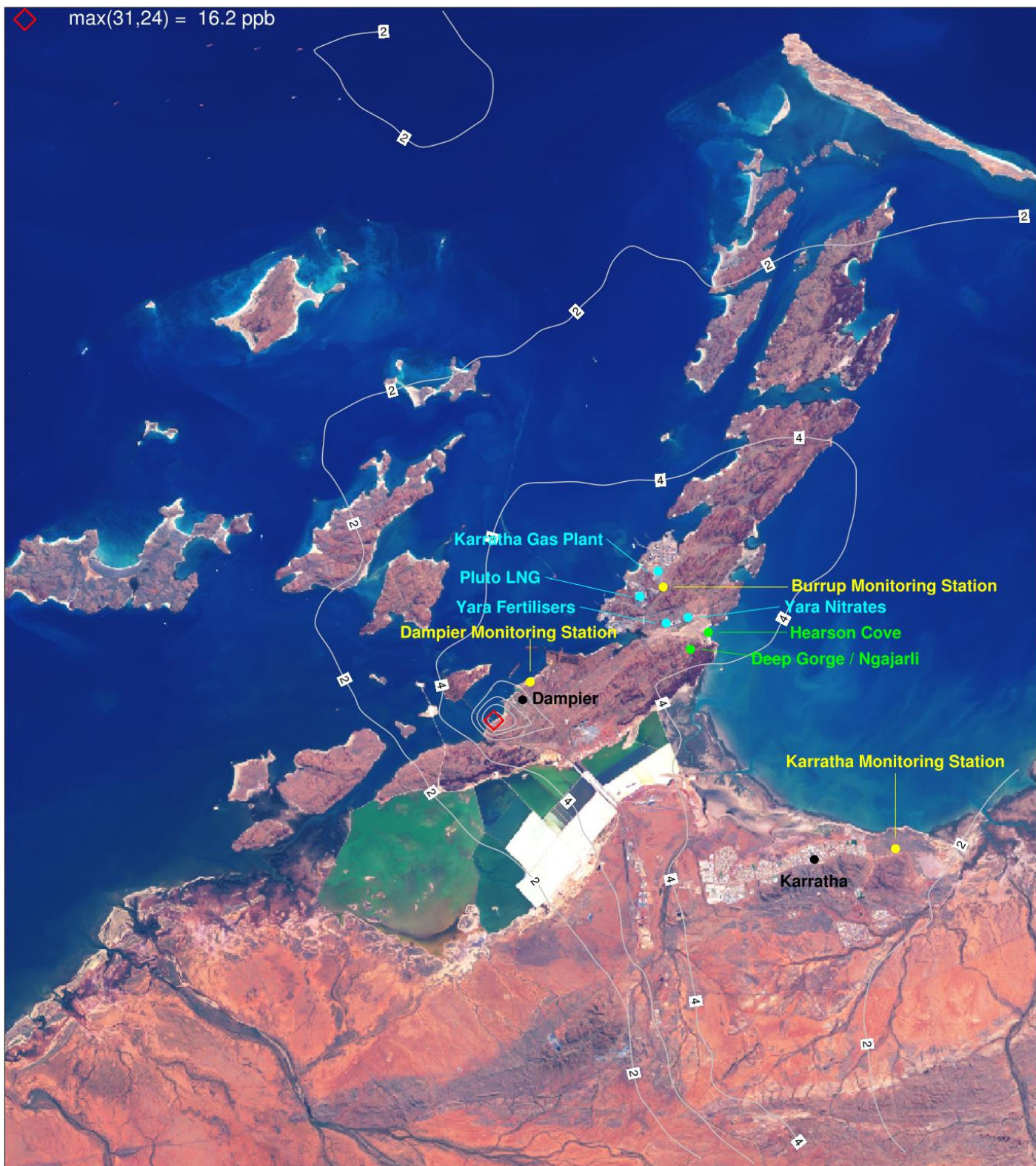
Figure 6-49. NO 2 (ppb) annual average ground level concentrations due to industry (S2-S1) for a subset of the CAMx 1.33 km domain centred over the Burrup Peninsula.
