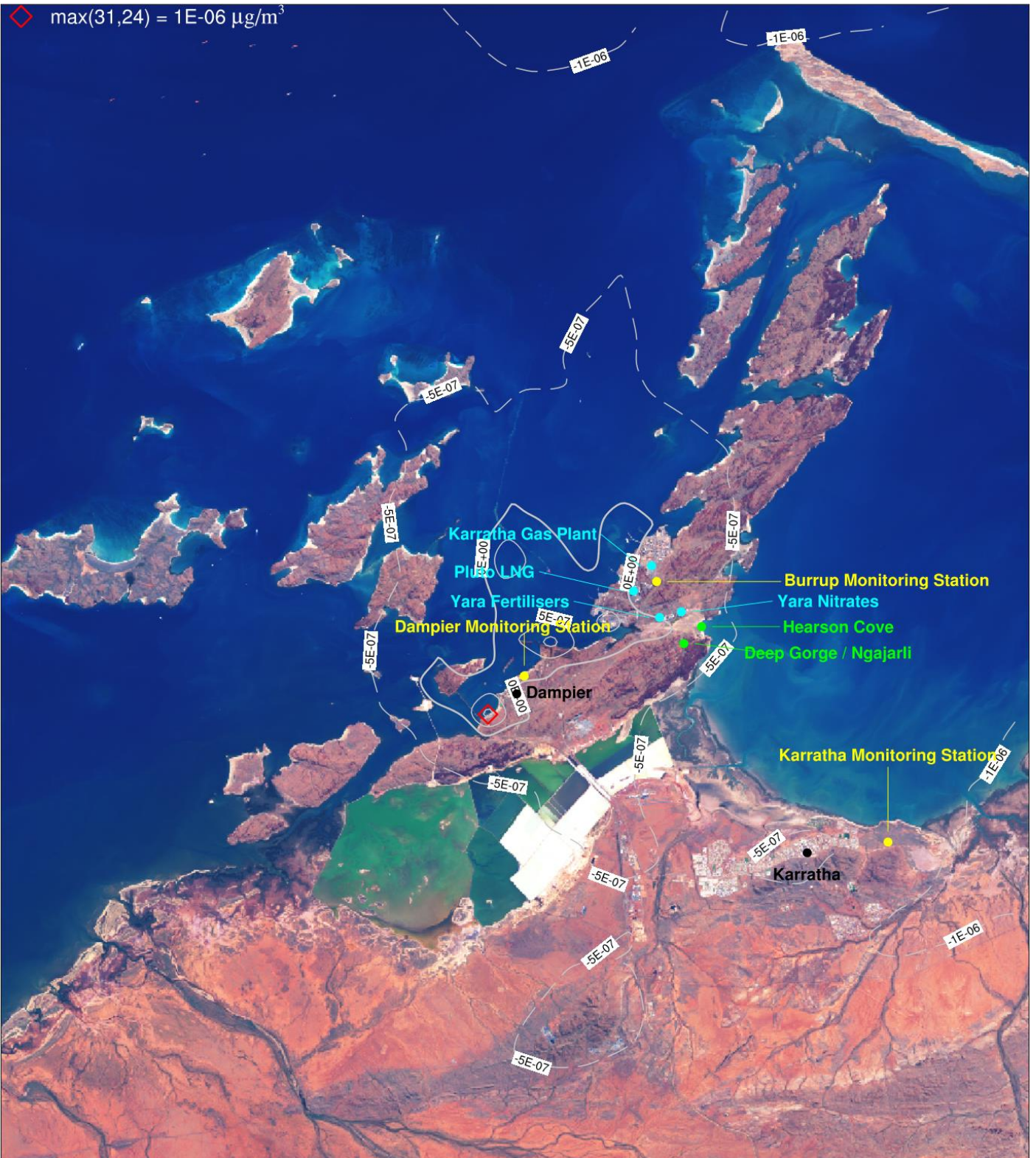
Figure 6-54. Hg ( \mu\text{g}/\text{m}^3 ) annual average ground level concentrations due to industry (S2-S1) for a subset of the CAMx 1.33 km domain centred over the Burrup Peninsula.
