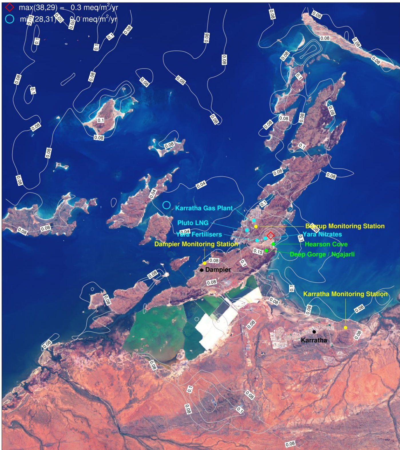
Figure 6-113. Annual total ammonium plus nitrate (meq/m 2 /yr) change in deposition from Scenario 2 due to future industry (S3-S2) for a subset of the CAMx 1.33 km domain centred over the Burrup Peninsula.
