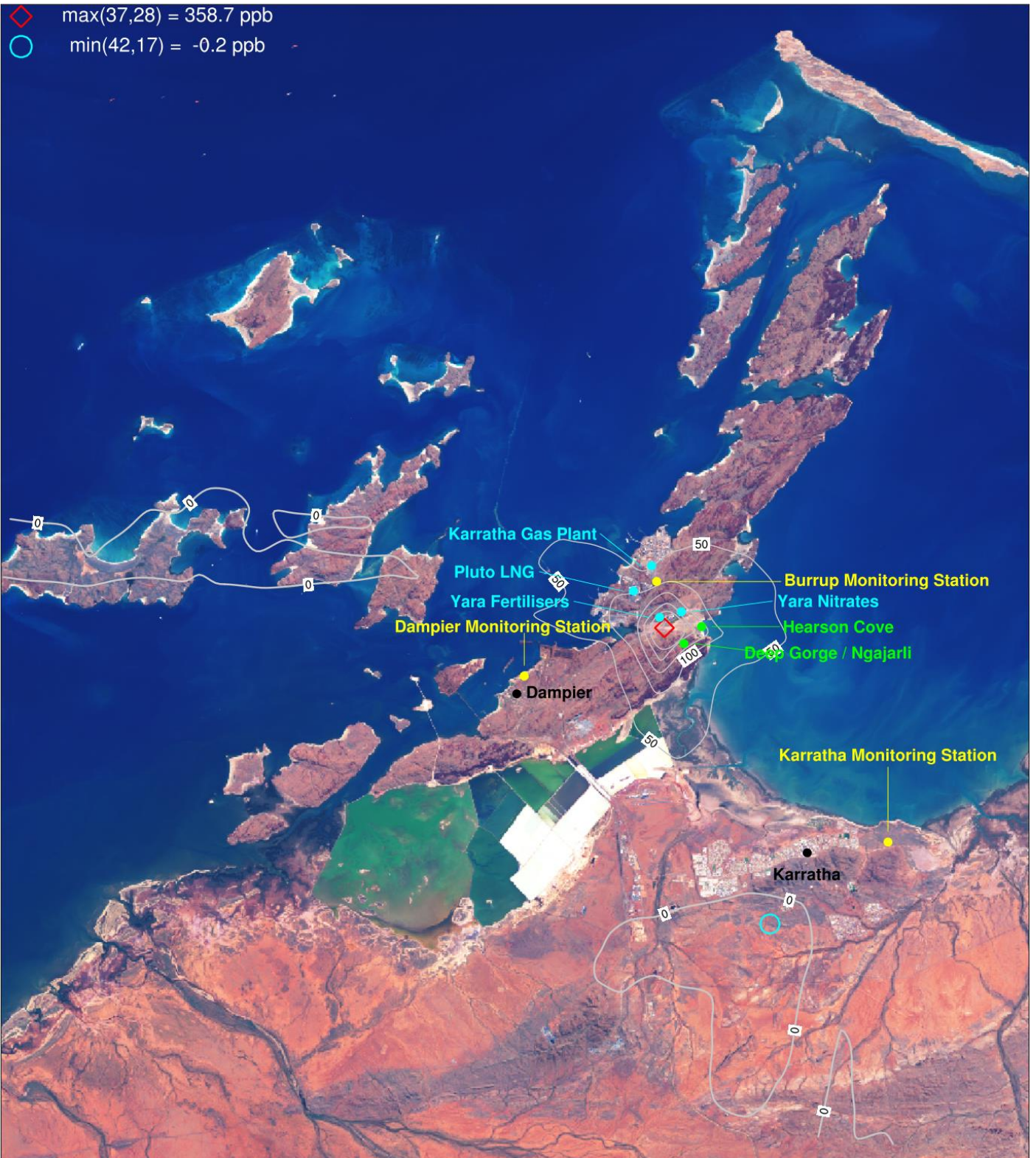
Figure 6-72. CO (ppb) change in annual max 8-hour (MDA8) ground level concentrations from Scenario 2 due to future industry (S3-S2) for a subset of the CAMx 1.33 km domain centred over the Burrup Peninsula.
