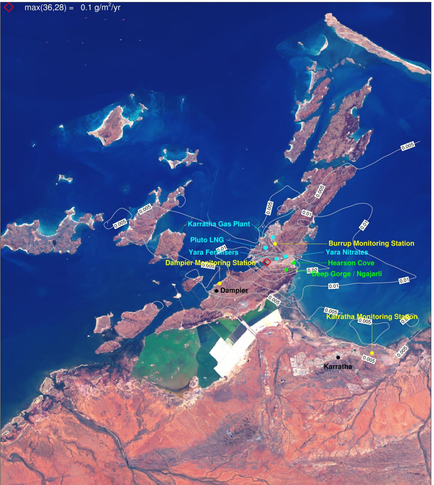
Figure 6-114. Annual total urea fine dust ( \text{g/m}^2/\text{yr} ) change in deposition from Scenario 2 due to future industry (S3-S2) for a subset of the CAMx 1.33 km domain centred over the Burrup Peninsula.
