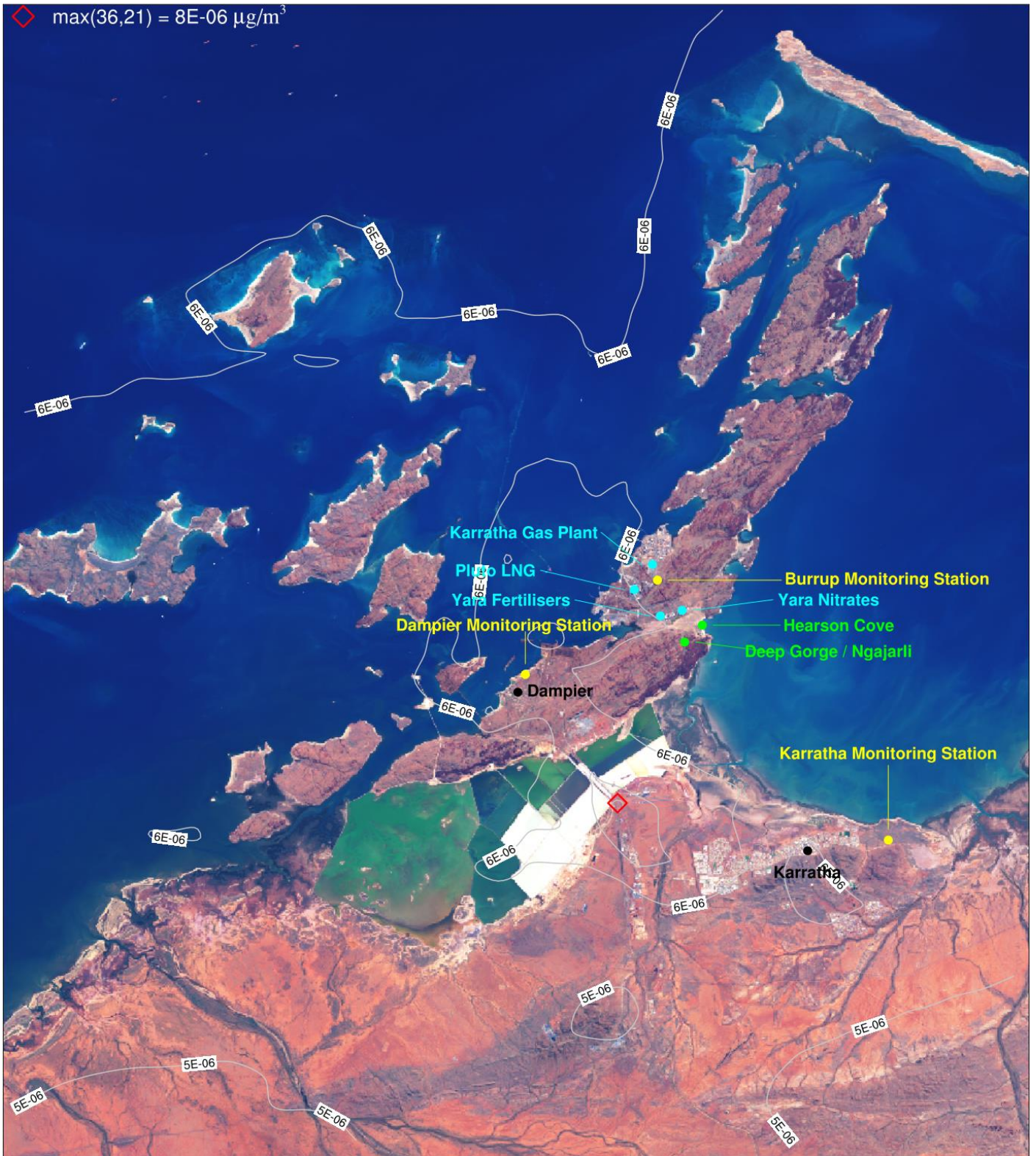
Figure 6-33. Hg ( \mu\text{g}/\text{m}^3 ) annual average concentrations for Scenario 2 (S2) for a subset of the CAMx 1.33 km domain centred over the Burrup Peninsula.
