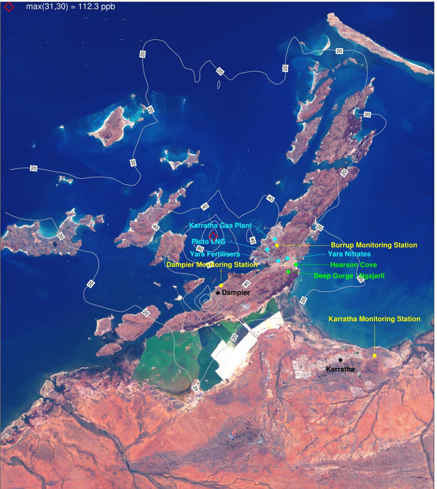
Figure 6-48. SO 2 (ppb) annual max 1-hour (MDA1) ground level concentrations due to industry (S2-S1) for a subset of the CAMx 1.33 km domain centred over the Burrup Peninsula.
