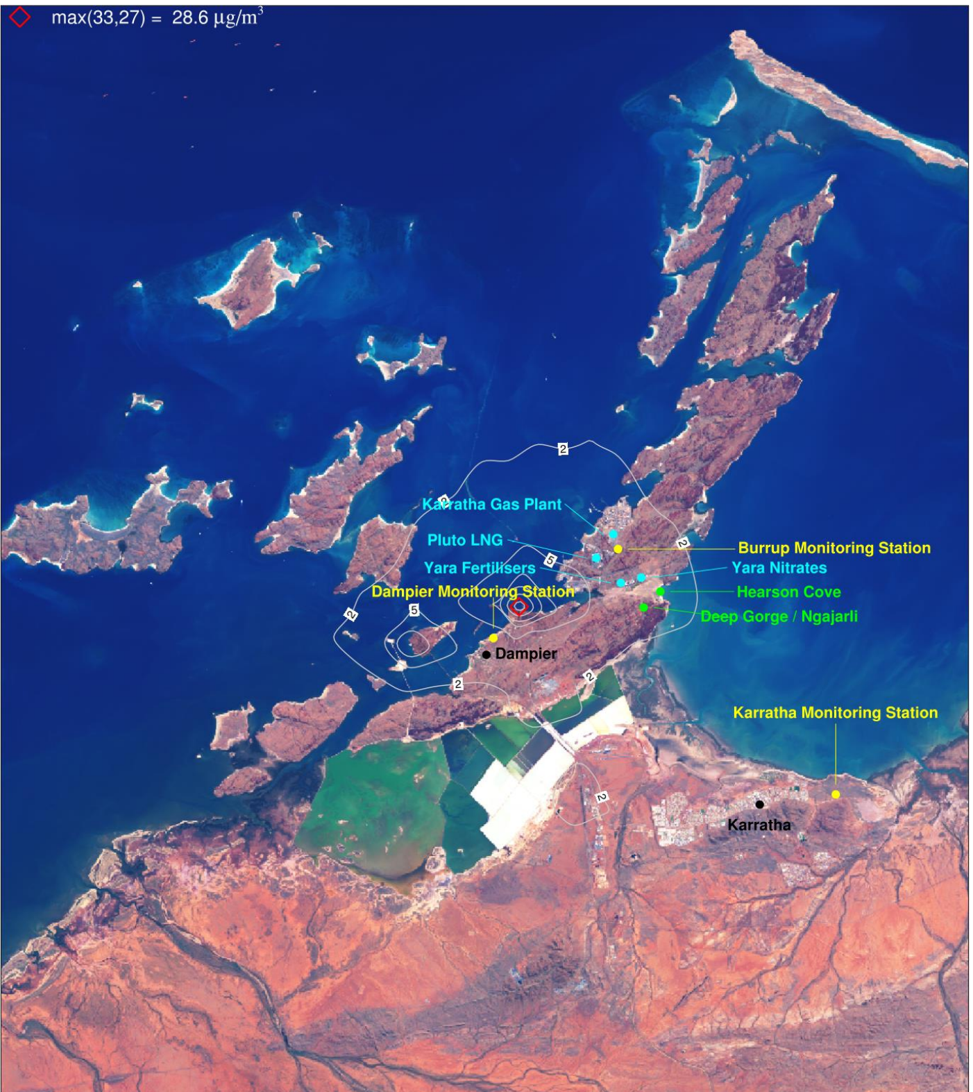
Figure 6-56. PM 10 ( \mu\text{g}/\text{m}^3 ) annual average ground level concentrations due to industry (S2-S1) for a subset of the CAMx 1.33 km domain centred over the Burrup Peninsula.
