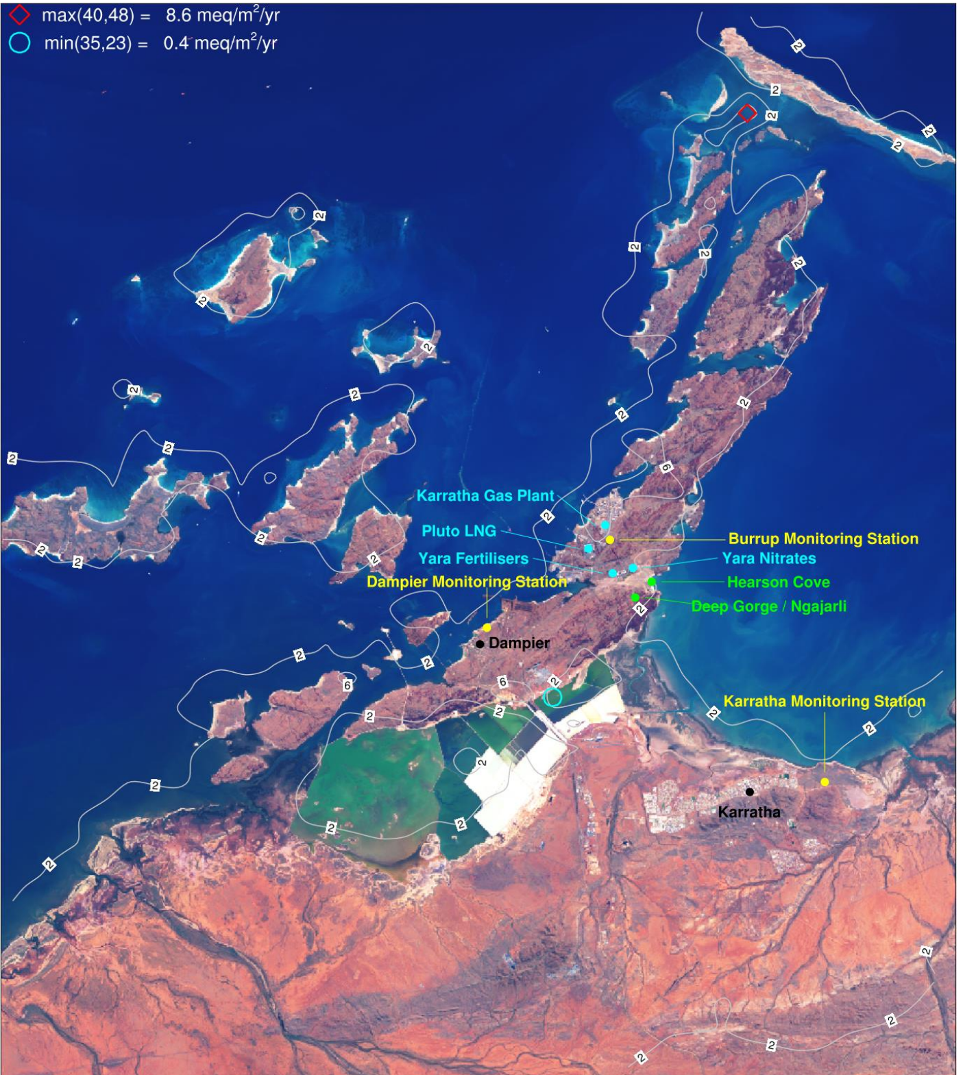
Figure 6-107. Annual total HNO 3 (nitric acid; units: meq/m 2 /yr) change in deposition from Scenario 2 due to future industry (S3-S2) for a subset of the CAMx 1.33 km domain centred over the Burrup Peninsula.
