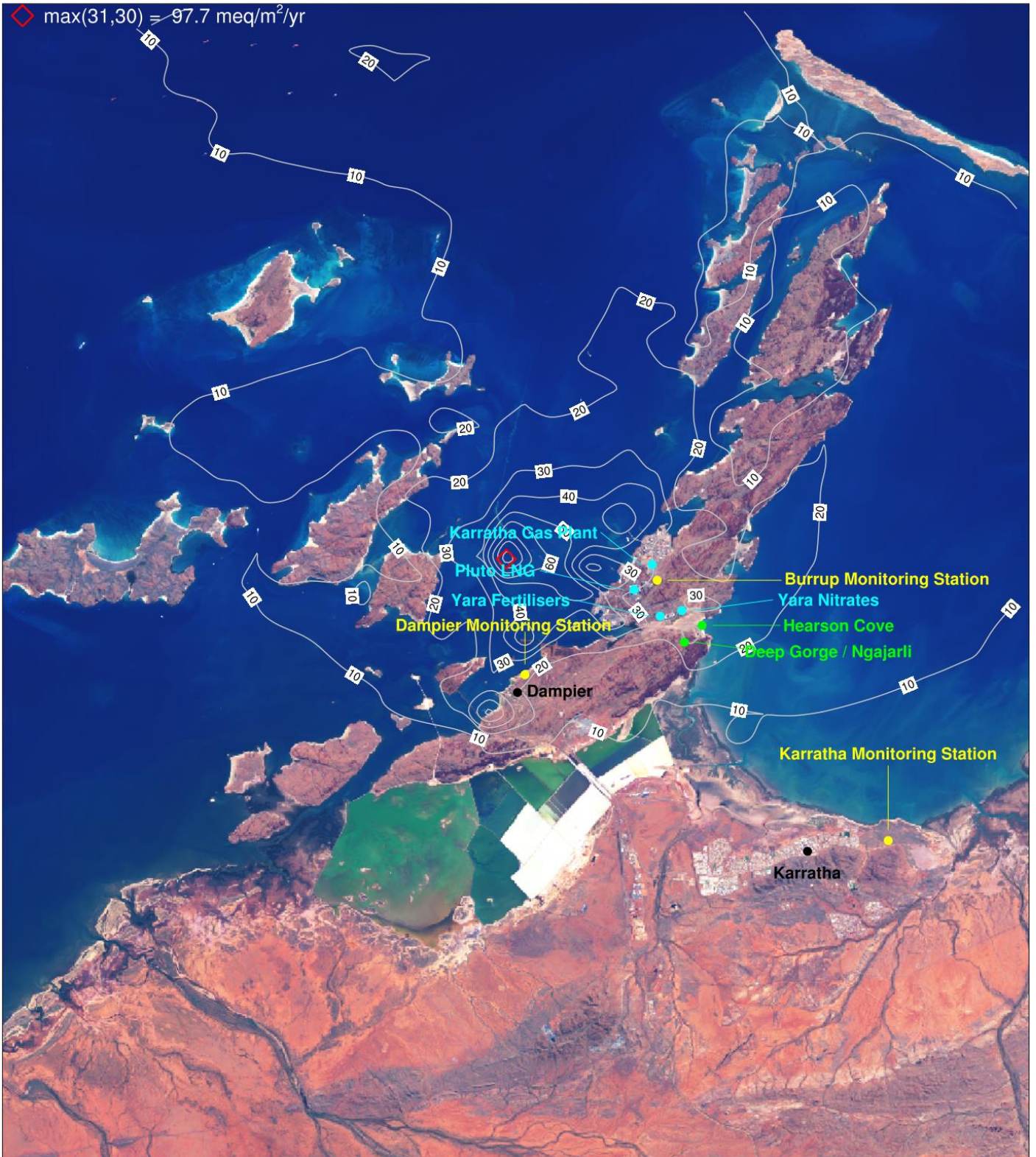
Figure 6-92. Annual total SO 2 (meq/m 2 /yr) deposition for Scenario 2 (S2) for a subset of the CAMx 1.33 km domain centred over the Burrup Peninsula.
