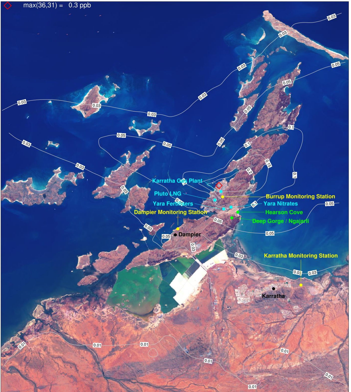
Figure 6-39. Benzene (ppb) annual average ground level concentrations due to industry (S2-S1) for a subset of the CAMx 1.33 km domain centred over the Burrup Peninsula.
