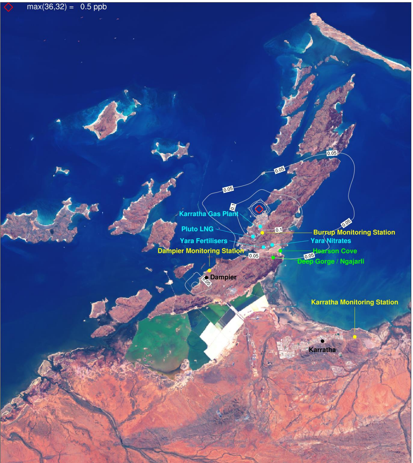
Figure 6-44. XYL (ppb) annual average ground level concentrations due to industry (S2-S1) for a subset of the CAMx 1.33 km domain centred over the Burrup Peninsula.
