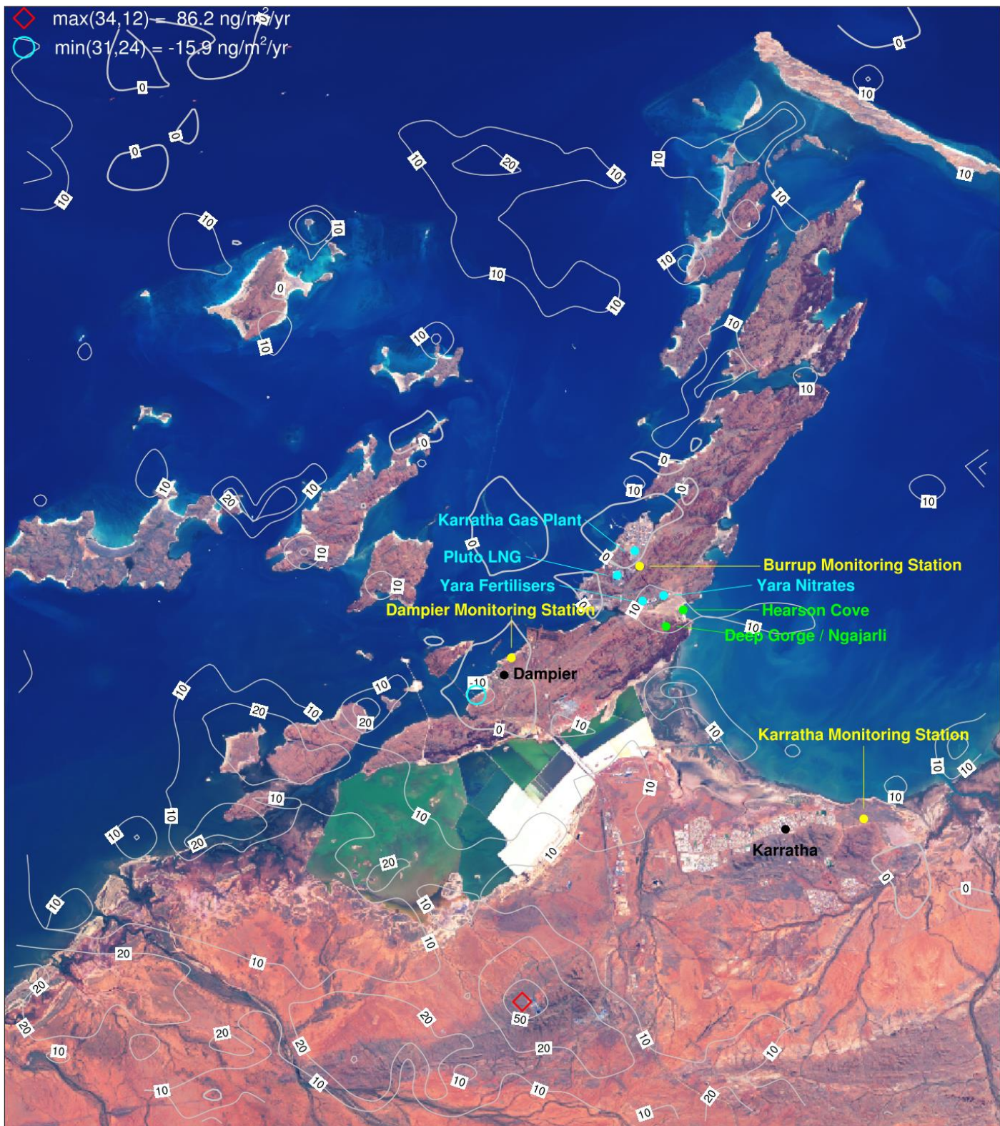
Figure 6-104. Annual total Hg (ng/m 2 /yr) change in deposition from Scenario 2 due to future industry (S3-S2) for a subset of the CAMx 1.33 km domain centred over the Burrup Peninsula.
