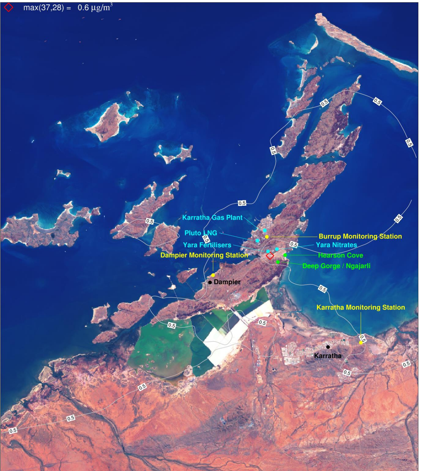
Figure 6-81. Ammonium plus nitrate ( \mu\text{g}/\text{m}^3 ) annual average concentrations for Scenario 2 (S2) for a subset of the CAMx 1.33 km domain centred over the Burrup Peninsula.
