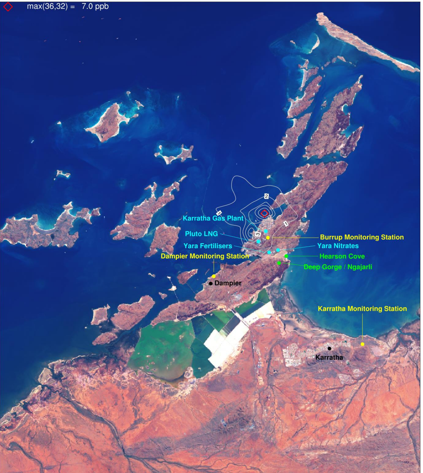
Figure 6-24. XYL (ppb) annual max 24-hour concentrations for Scenario 2 (S2) for a subset of the CAMx 1.33 km domain centred over the Burrup Peninsula.
