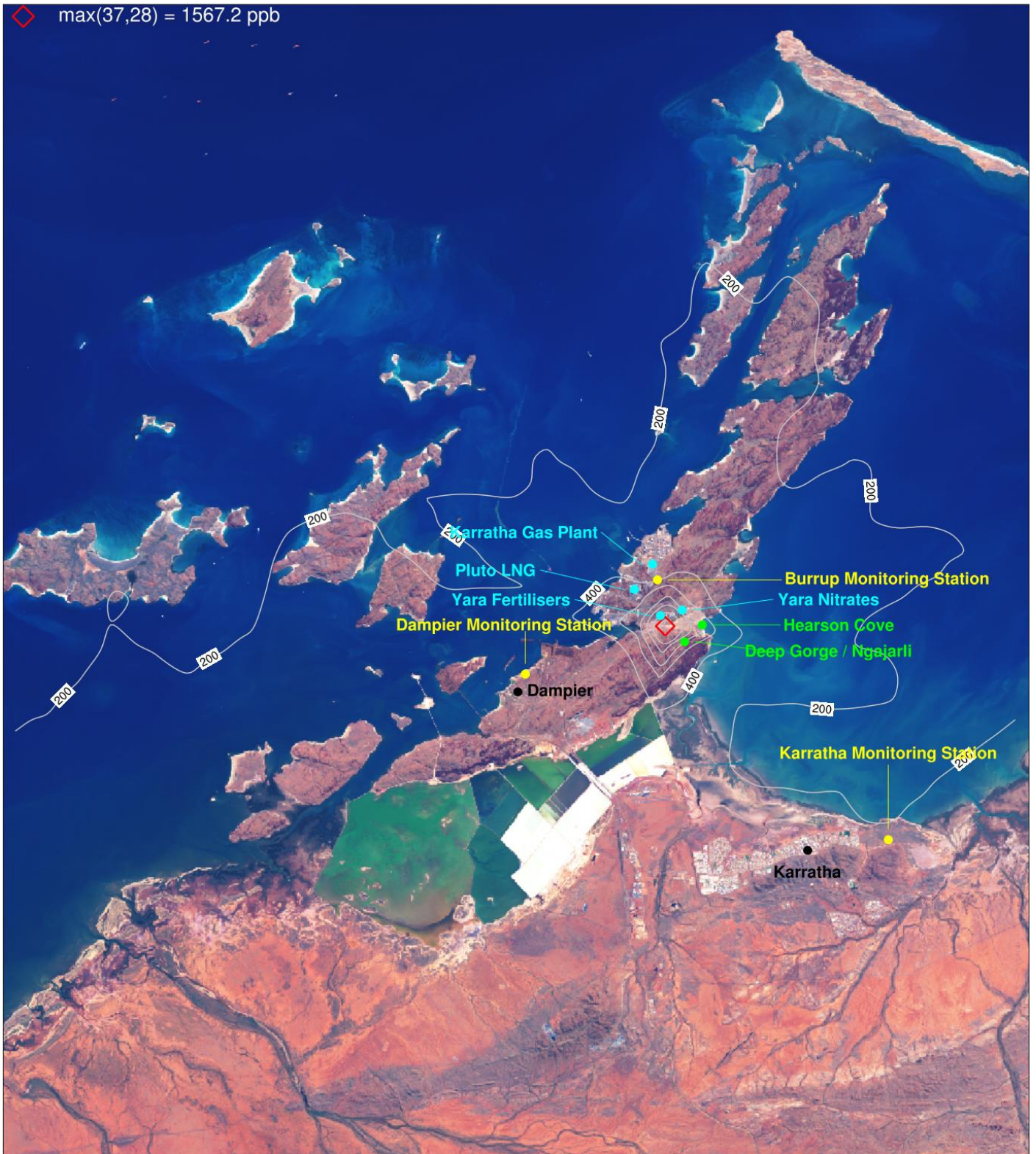
Figure 6-30. CO (ppb) annual max 8-hour (MDA8) concentrations for Scenario 2 (S2) for a subset of the CAMx 1.33 km domain centred over the Burrup Peninsula.
