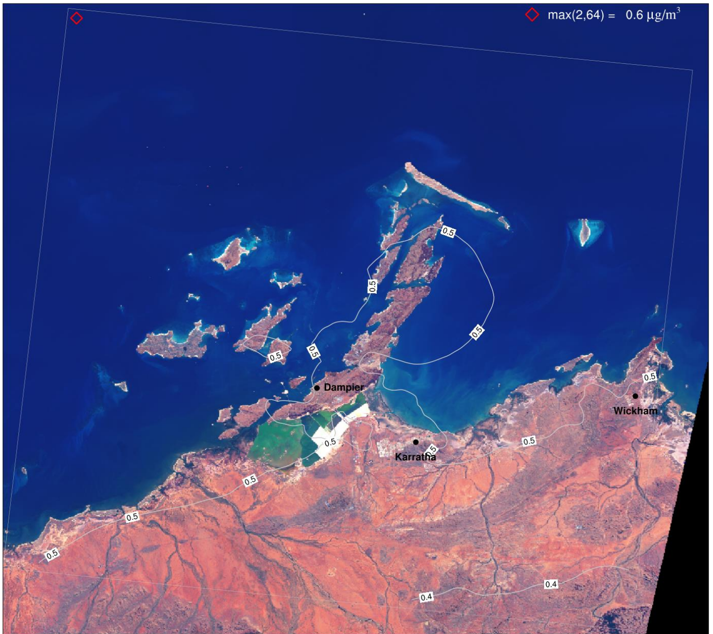
Figure A2-22. Ammonium plus nitrate ( \mu\text{g}/\text{m}^3 ) annual average concentrations for Scenario 2 (S2) for the CAMx 1.33 km domain.
