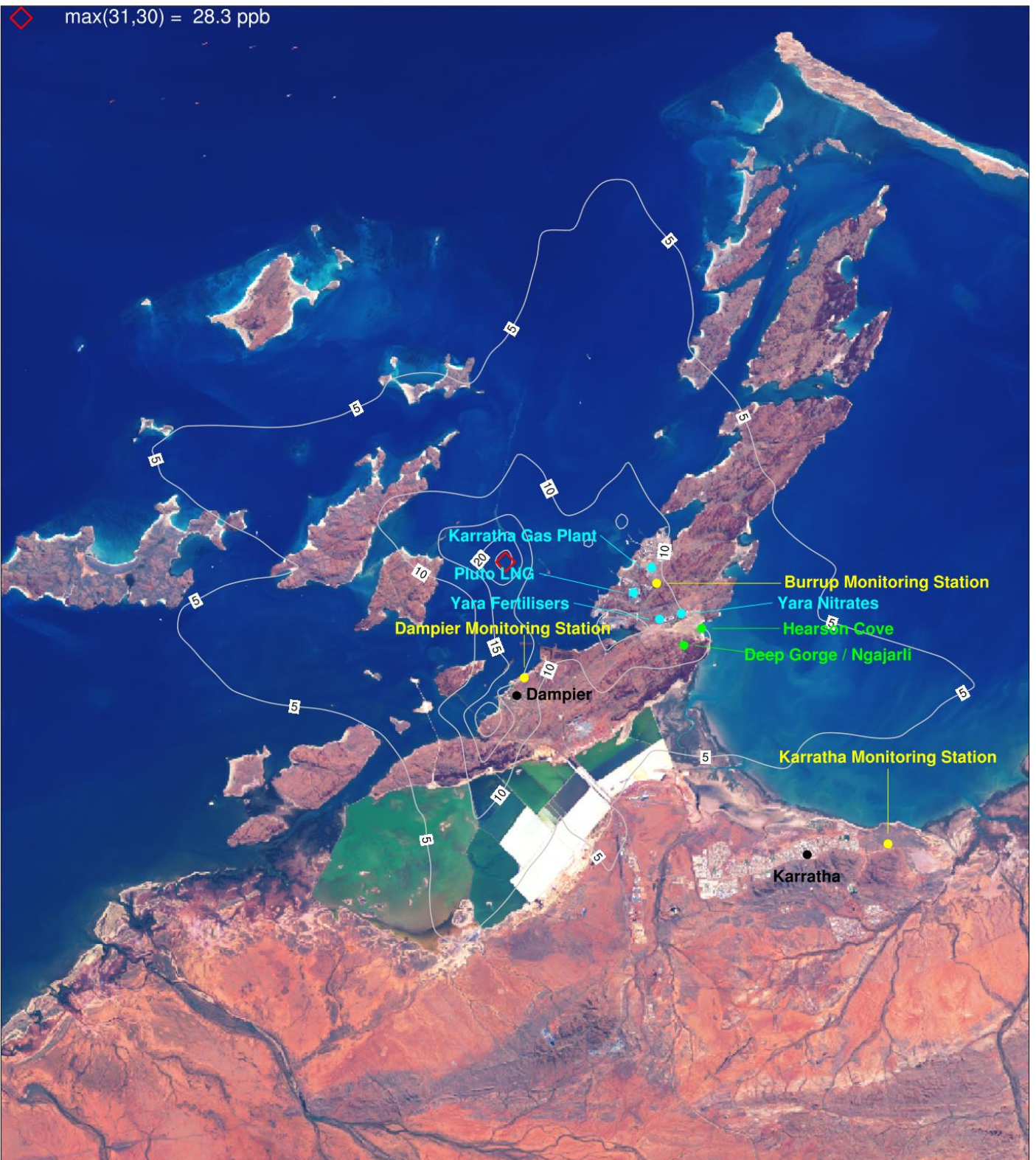
Figure 6-47. SO 2 (ppb) annual max 24-hour ground level concentrations due to industry (S2-S1) for a subset of the CAMx 1.33 km domain centred over the Burrup Peninsula.
