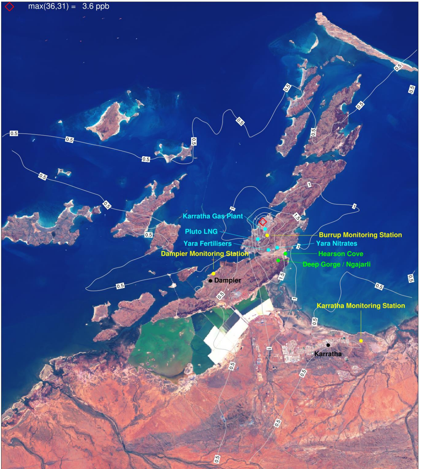
Figure 6-21. TOL (ppb) annual max 24-hour concentrations for Scenario 2 (S2) for a subset of the CAMx 1.33 km domain centred over the Burrup Peninsula.
