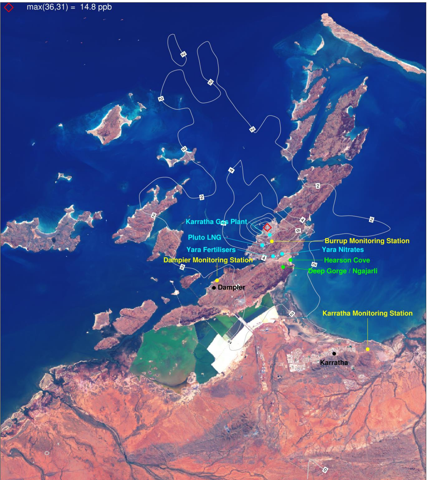
Figure 6-40. Benzene (ppb) annual max 1-hour (MDA1) ground level concentrations due to industry (S2-S1) for a subset of the CAMx 1.33 km domain centred over the Burrup Peninsula.
