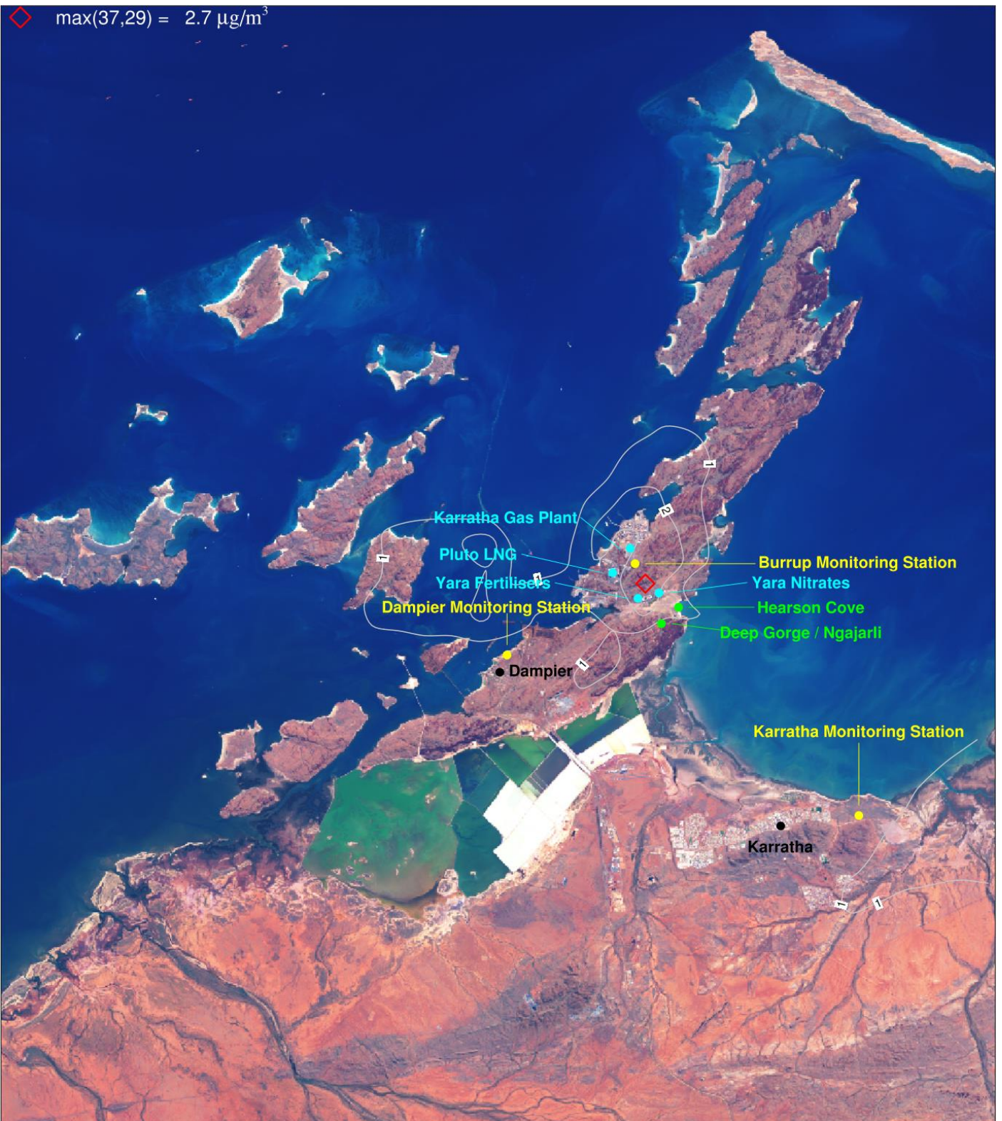
Figure 6-59. PM 2.5 ( \mu\text{g}/\text{m}^3 ) annual max 24-hour ground level concentrations due to industry (S2-S1) for a subset of the CAMx 1.33 km domain centred over the Burrup Peninsula.
