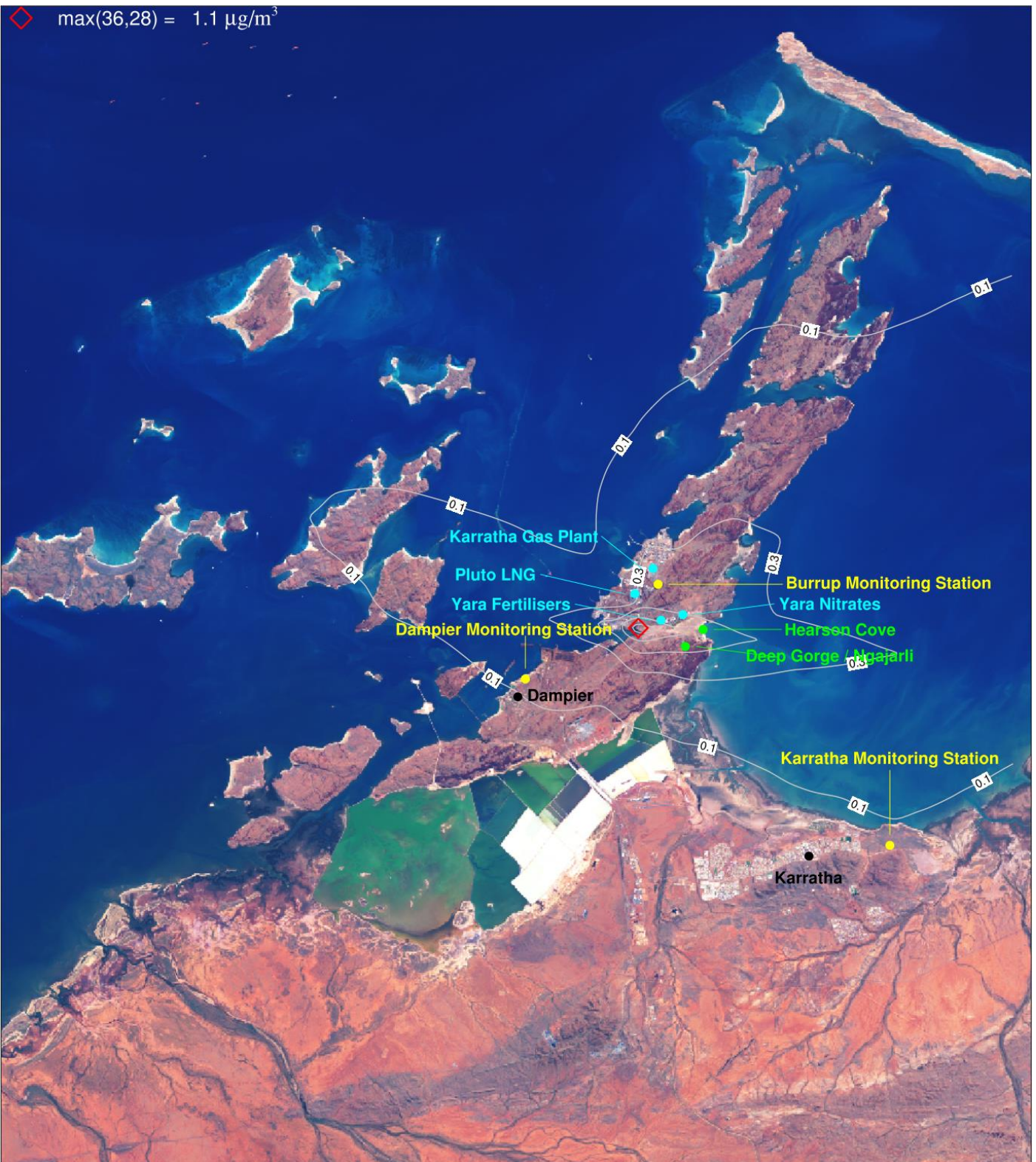
Figure 6-84. Urea fine dust ( \mu\text{g}/\text{m}^3 ) change in annual average ground level concentrations from Scenario 2 due to future industry (S3-S2) for a subset of the CAMx 1.33 km domain centred over the Burrup Peninsula.
