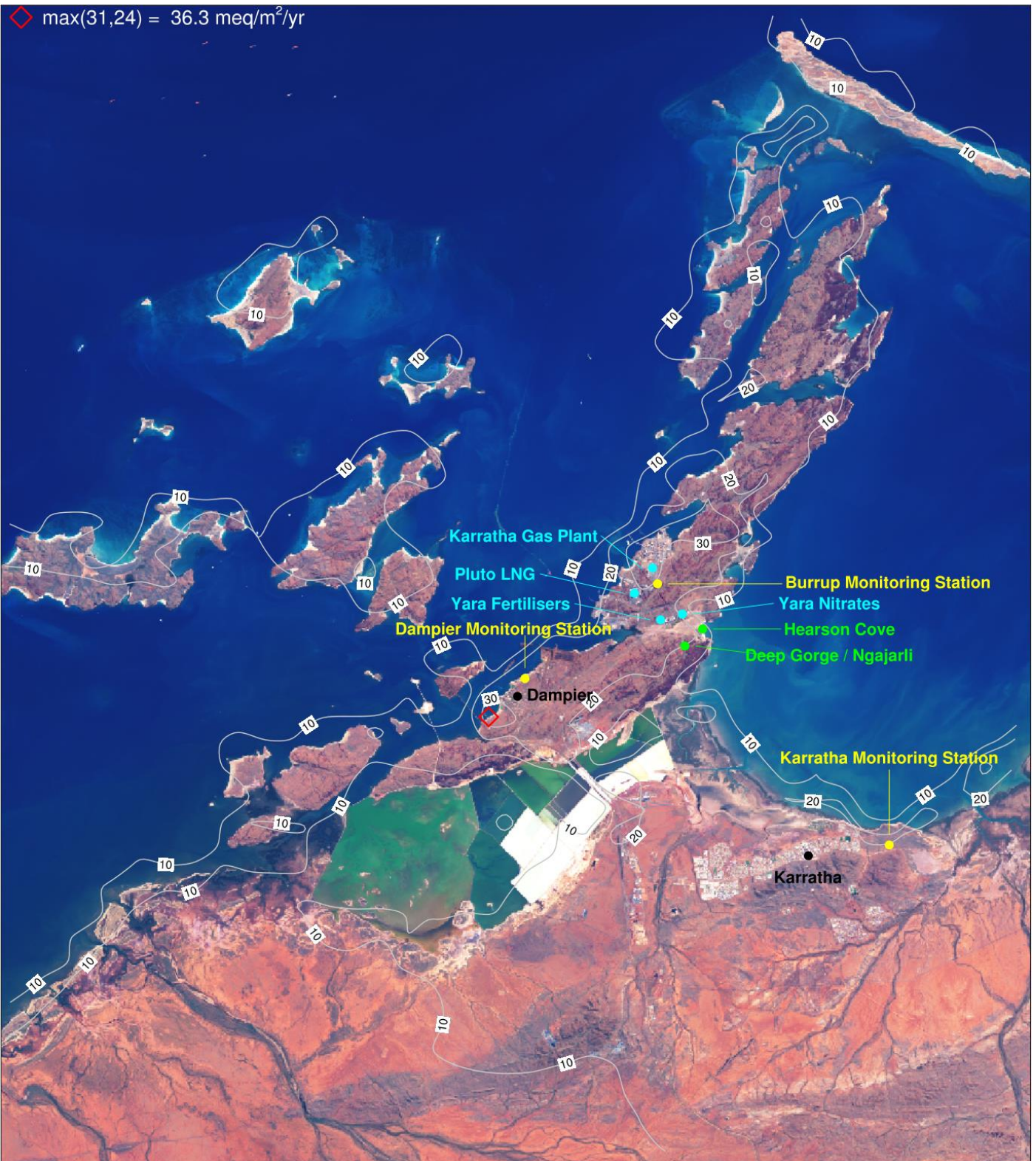
Figure 6-90. Annual total N (nitrogen; units: meq/m 2 /yr) deposition for Scenario 2 (S2) for a subset of the CAMx 1.33 km domain centred over the Burrup Peninsula.
