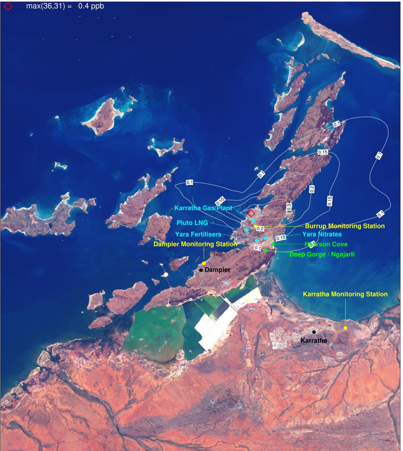
Figure 6-41. TOL (ppb) annual average ground level concentrations due to industry (S2-S1) for a subset of the CAMx 1.33 km domain centred over the Burrup Peninsula.
