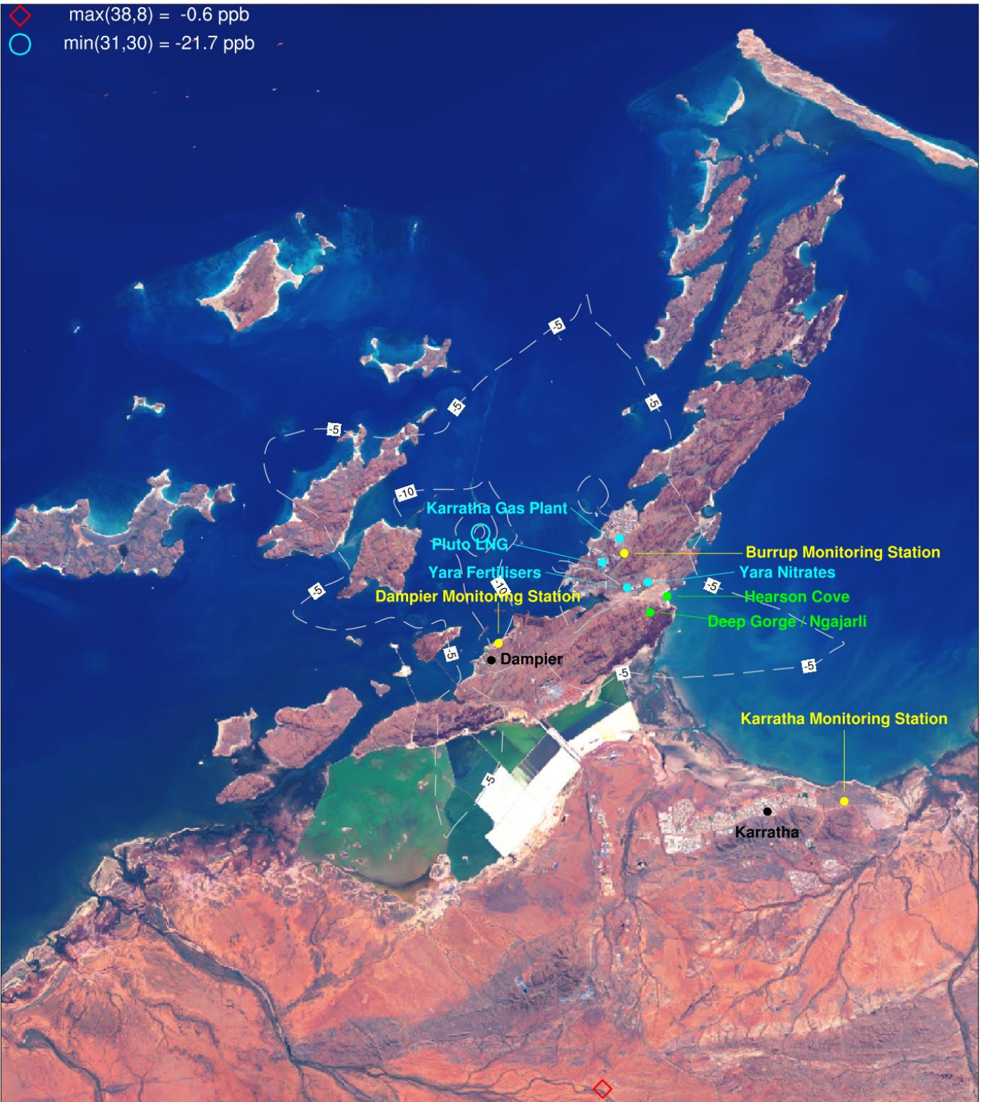
Figure 6-68. SO 2 (ppb) change in annual max 24-hour ground level concentrations from Scenario 2 due to future industry (S3-S2) for a subset of the CAMx 1.33 km domain centred over the Burrup Peninsula.
