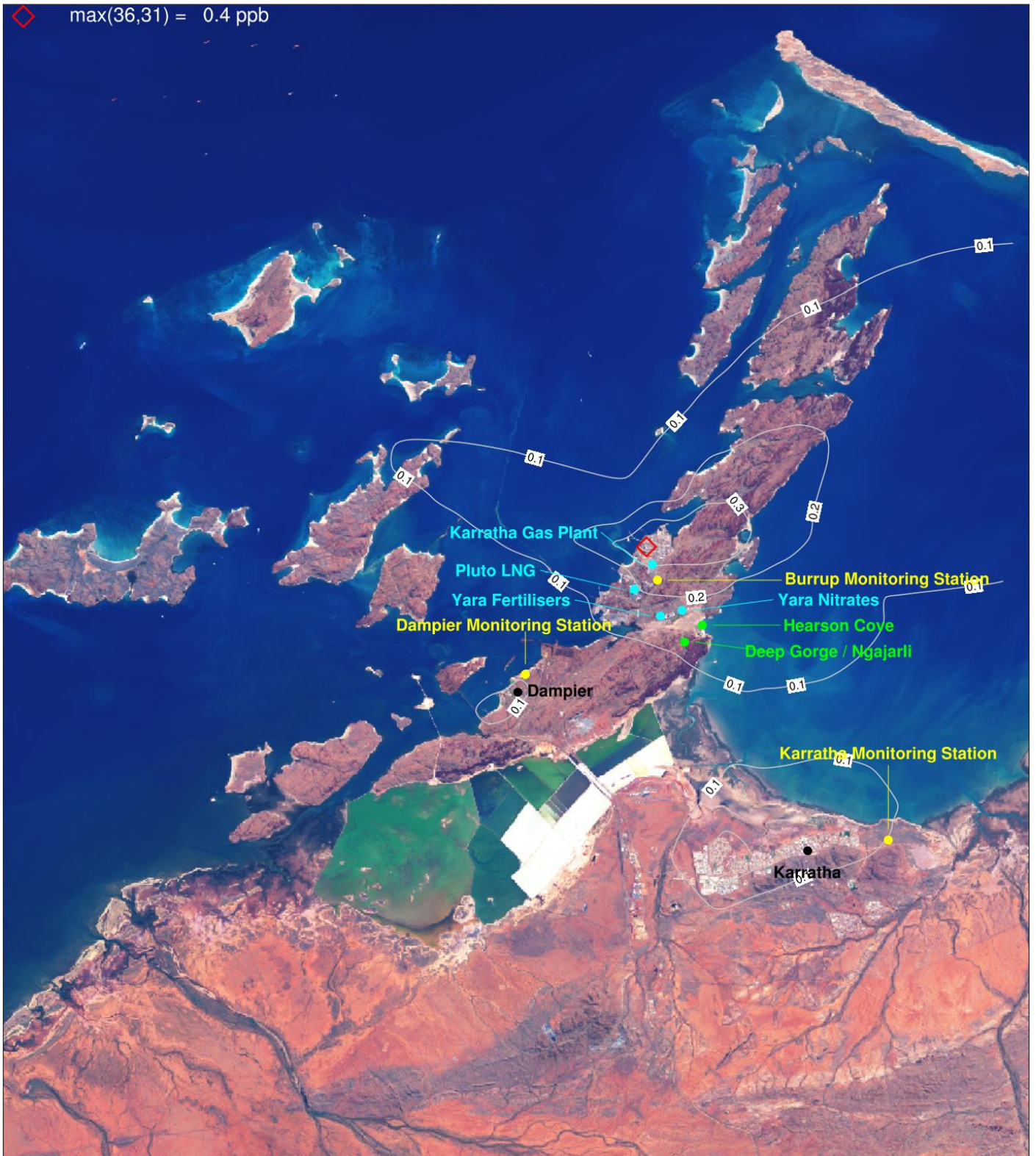
Figure 6-20. TOL (ppb) annual average concentrations for Scenario 2 (S2) for a subset of the CAMx 1.33 km domain centred over the Burrup Peninsula.
