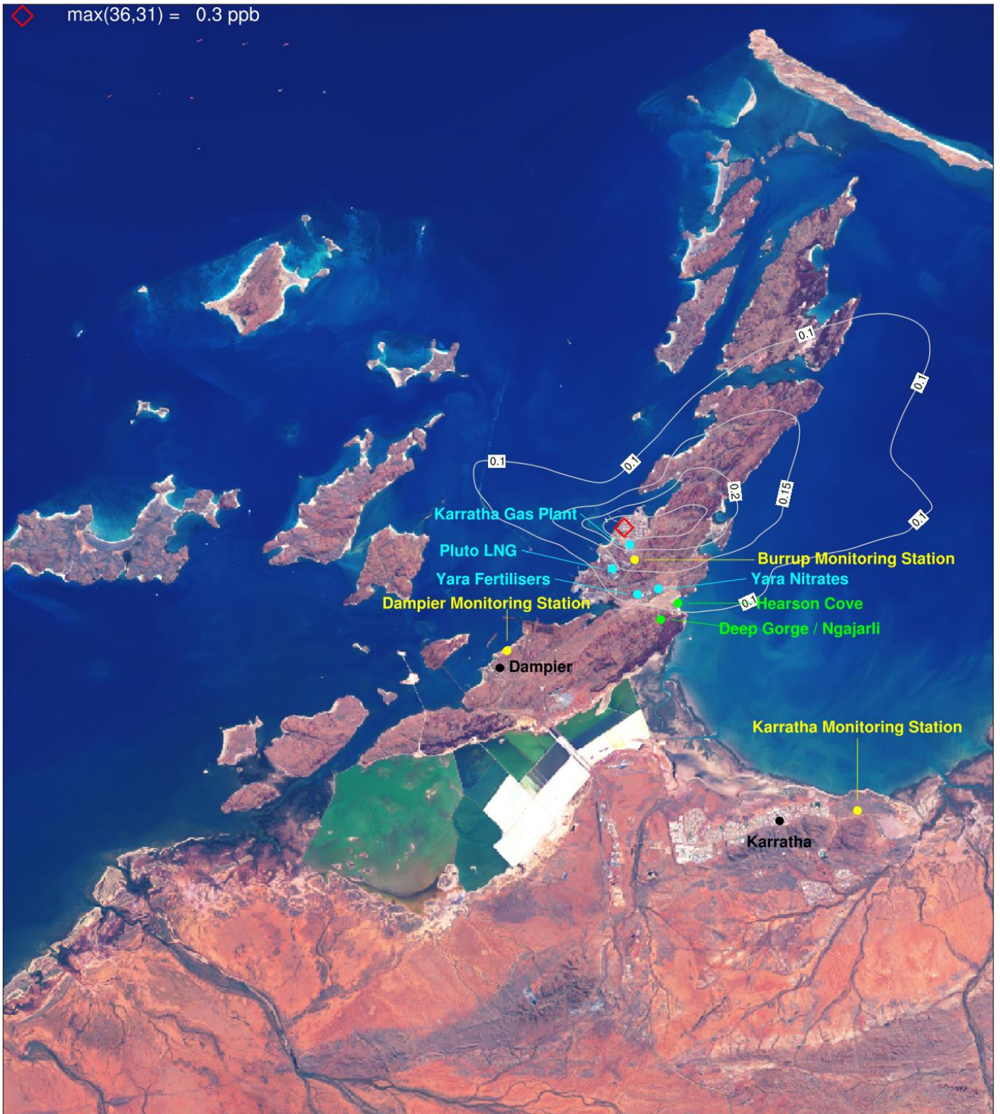
Figure 6-18. Benzene (ppb) annual average concentrations for Scenario 2 (S2) for a subset of the CAMx 1.33 km domain centred over the Burrup Peninsula.
