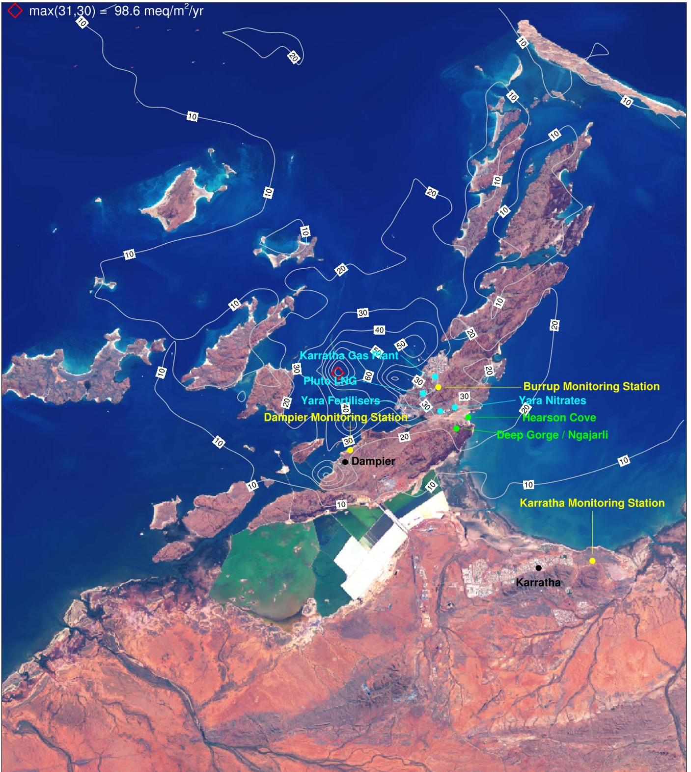
Figure 6-93. Annual total S (sulphur; units: meq/m 2 /yr) deposition for Scenario 2 (S2) for a subset of the CAMx 1.33 km domain centred over the Burrup Peninsula.
