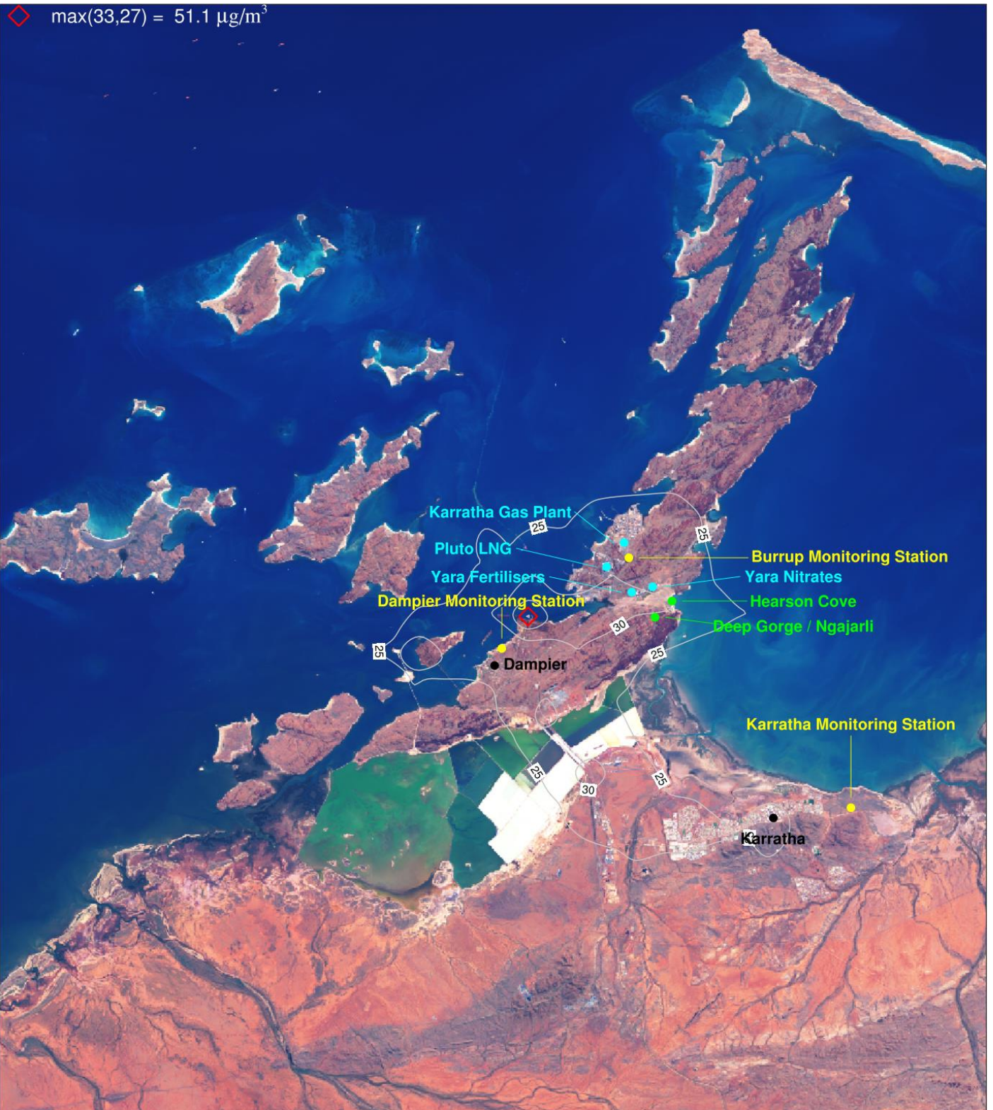
Figure 6-35. PM 10 ( \mu\text{g}/\text{m}^3 ) annual average concentrations for Scenario 2 (S2) for a subset of the CAMx 1.33 km domain centred over the Burrup Peninsula.
