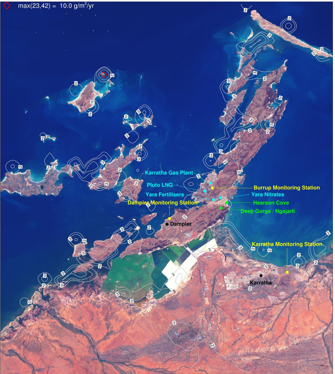
Figure 6-86. Annual total dust ( \text{g/m}^2/\text{yr} ) deposition for Scenario 2 (S2) for a subset of the CAMx 1.33 km domain centred over the Burrup Peninsula.
