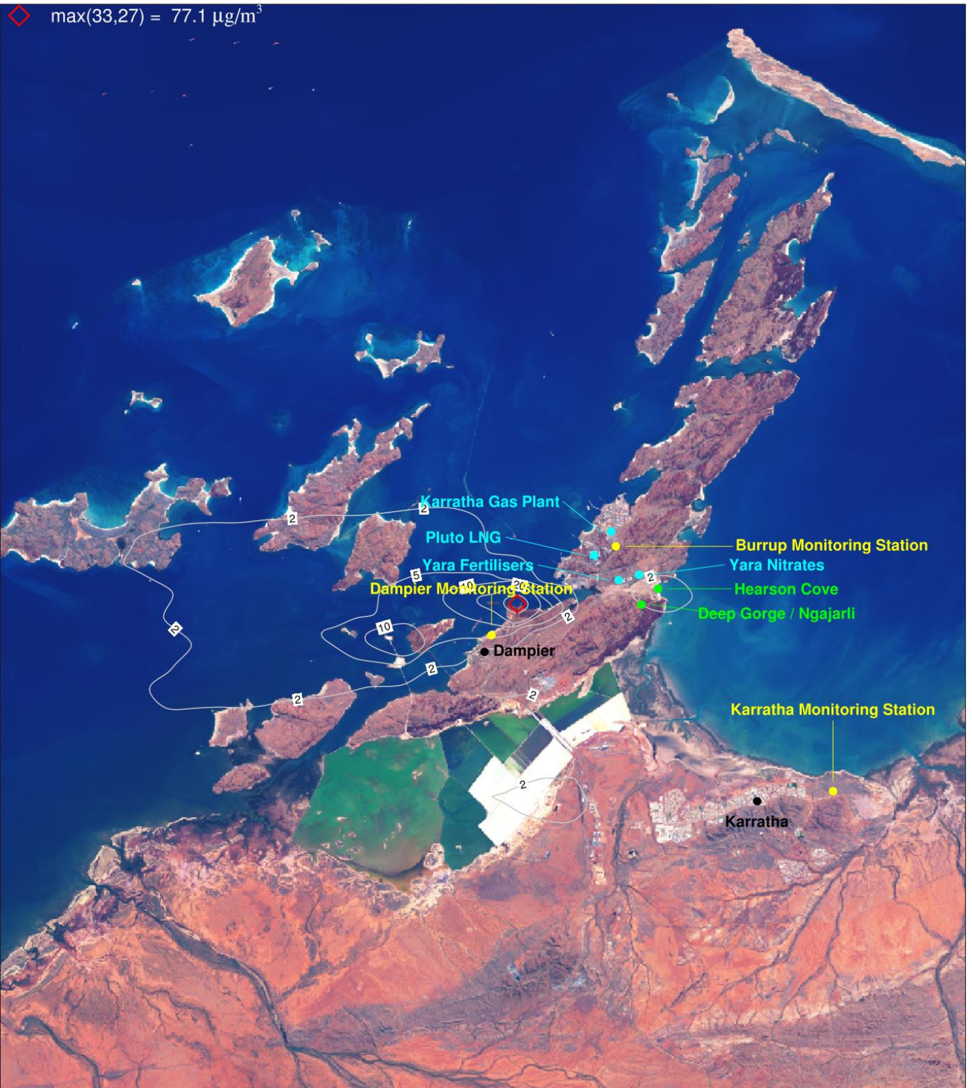
Figure 6-57. PM 10 ( \mu\text{g}/\text{m}^3 ) annual max 24-hour ground level concentrations due to industry (S2-S1) for a subset of the CAMx 1.33 km domain centred over the Burrup Peninsula.
