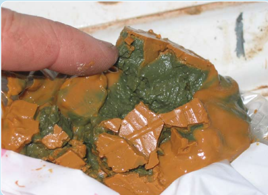
Figure 3 Iron and aluminium rich sludge precipitated from drain water after neutralisation with hydrated lime
