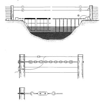
Figure 10: Electrified flood gate.
