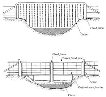
Figure 9: Fixed frame flood gate.
