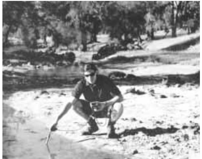
Testing the salinity of the Warperup Creek, a tributary of the Pallinup River. This was part of a floodway condition assessment carried out in late 2001.
