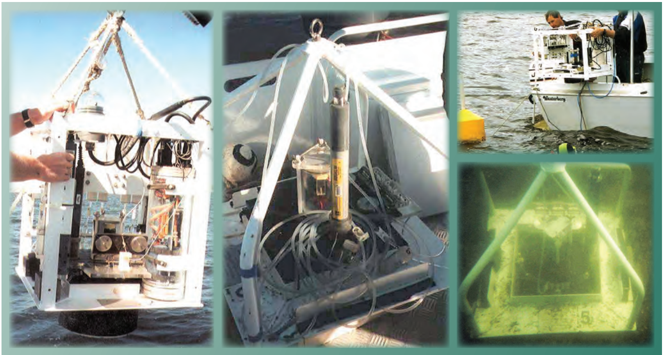
Figure 8. Manual and automatic benthic chambers, underwater and being deployed.
