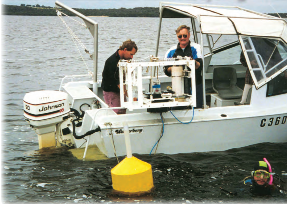
Figure 1. Deploying a benthic chamber in Wilson Inlet to measure sediment nutrient fluxes.
