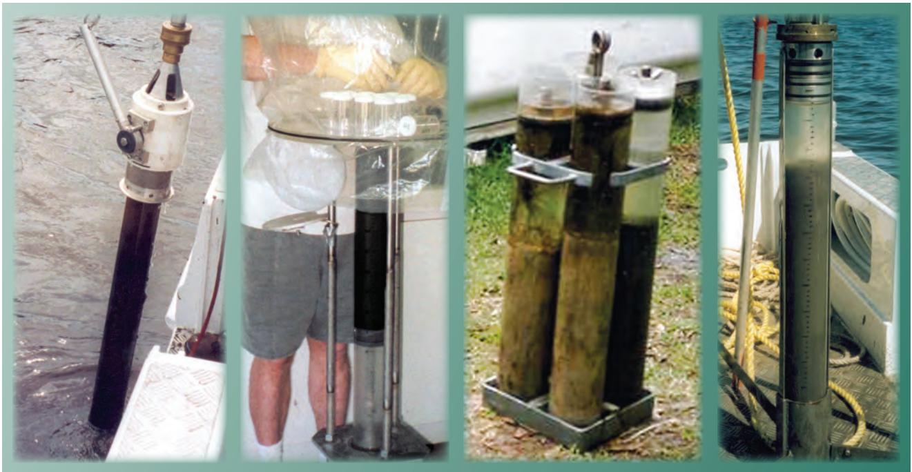
Figure 4. Sediment cores being collected and then extruded under nitrogen gas (so that the sediments and pore-waters are not exposed to atmospheric oxygen). Note the difference between dark muddy sediments and light-coloured sandy sediments. Photos: B. Boardman
